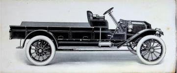
In express or delivery wagon style the Model 820 has all the advantages as in the Mountain Wagon style. The ease of control and absence of clutch and gear-shift make it very desirable for routes with frequent stops; and the absence of engine vibration makes the car adaptable to carrying garden produce to market and transporting other kinds of perishable goods.
