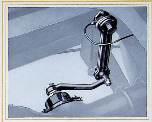
Both front and rear shock absorbers are two-way in their action and make possible the use of much more resilient springs, the riding adjustment being made in the shock absorbers.
