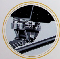
The rear of the left front spring is provided with a shock-absorbing device.
