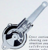
The shock absorbers on the Packard Eight are Packard in design and manufacture and are found on no other car. They are not an addition to the chassis but rather an integral part of it.
