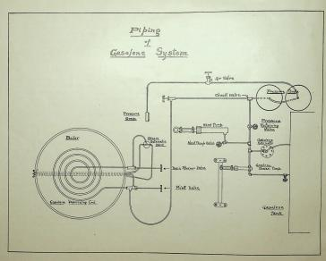
If the fire were now lighted, and allowed to burn for some time, the gasolene pressure would gradually drop. But it would only be necessary to use the hand gasolene pump to raise it again.
