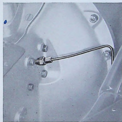
The clutch bearing is automatically oiled
