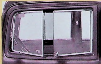
Front windows are simply operated for quick signalling and any degree of draft-free ventilation
