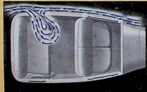
NEW: Swinging out the rear quarter window can confine the air flow to the rear seat only
