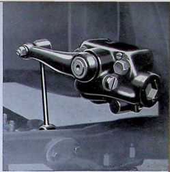
Shock absorbers are double-action hydraulic
