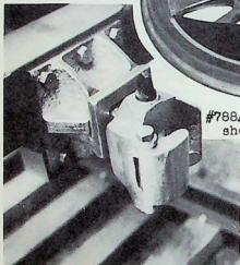
Application of Coupler and Draw bar Pocket. 3/4" scale castings, #7850 and #786.
