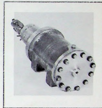
Drive Brake cylinder & heads, parts #BKE13-27, 28 & 29. Shown finished and assembled.
