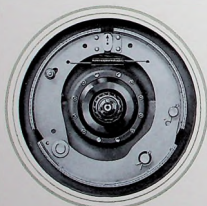
Brakes are self-energizing and but slight pedal pressure is required to produce utmost efficiency in even the coldest weather.
