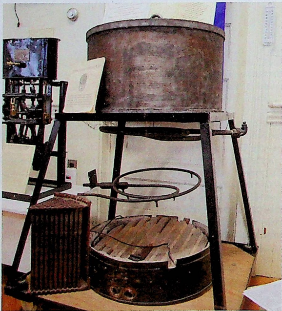
A steam boiler rests atop this display frame, with its burner below. The wedge-shaped piece to the left of the burner is a section of the boiler, showing the tubes incorporated in its construction.
