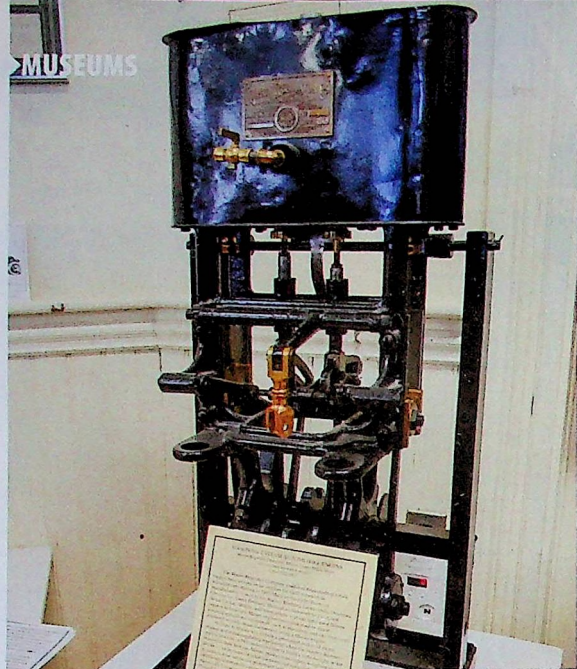
This is an example of the "Whitney-type" steam car engine that inspired the Stanleys. It was taken from an 1899 Locomobile steam carriage.
