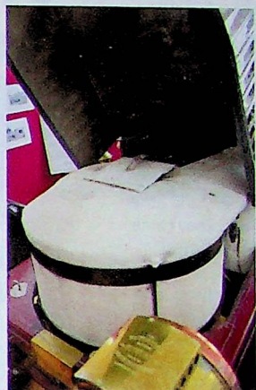
The boiler of the 1909 Stanley takes up nearly all of the room under the hood.
