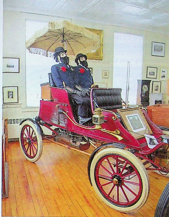
Mannequins dressed as F.E. and F.O. are posed in a 1905 Stanley Model CX. This would be the last year of production for tiller-steered cars, and the first year of the "coffin-nosed" models. Its 8-horsepower rating was based on its 16-inch-high boiler.
