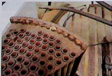
A steam boiler rests atop this display frame, with its burner below. The wedge-shaped piece to the left of the burner is a section of the boiler, showing the tubes incorporated in its construction.
