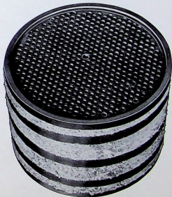
Stanley boiler. The shell and the lower head are of one piece, of pressed steel. The upper head, shell, and ring are welded together by the oxyacetylene process. The tubes are of copper, reinforced at each end with steel bushings. The bands indicated in the cut are of thin brass, to hold in place the half-inch sheet asbestos insulation.
