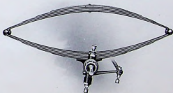
Front spring and spindle construction, showing how the spindle is set at an angle, to assist in easy steering
