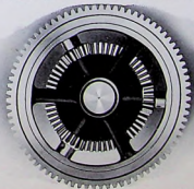
Detail showing Stanley differential and driving gear. The main driving gear, with its three beveled pinions, and one driving shaft with its bevel gear, are shown
