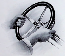
Steering wheel with hands, showing how the throttle lever is lightly gripped in the fingers without removing the hand from the wheel
