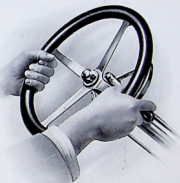
Steering wheel, with hands, showing how the throttle-lever is lightly gripped in the fingers without removing the hand from the wheel.
