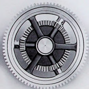
Detail showing Stanley differential and driving gear. The main driving gear with its three bevel pinions, and one driving shaft with its bevel gear, are shown.
