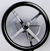
Steering wheel, showing the single throttle in the Stanley system of control locked by its locking screw ; and the by-pass lever.
