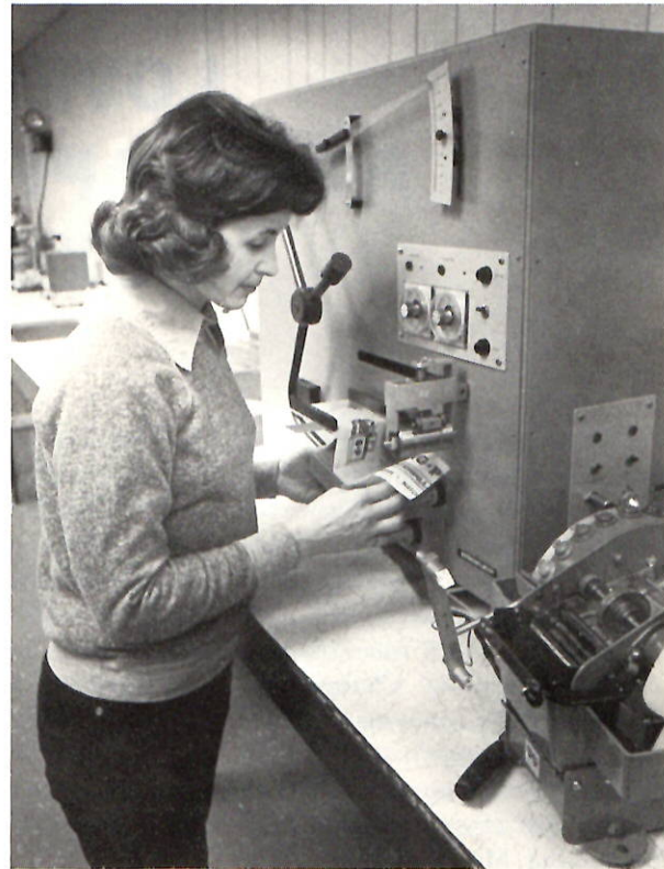
Shows portion of extensive inplant testing laboratory. Device shown is used for routine quality control testing of adhesive properties of gummed tapes.
