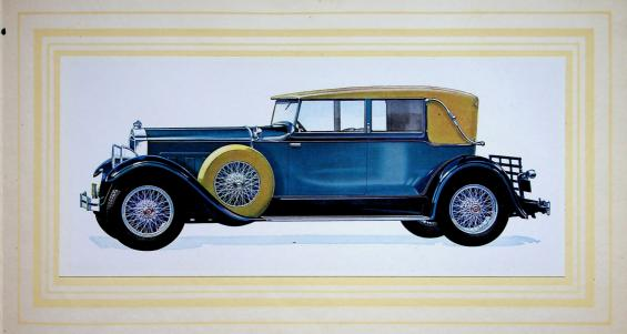
CHE new telescoping feature of the top design allows it to be folded compactly at an angle that blends with the streamline effect achieved by such details as the slanting windshield and molding treatment. The center pillar posts which hold the top rigid and serve as channels for the operation of door and body windows, fold entirely out of sight with the top down.
