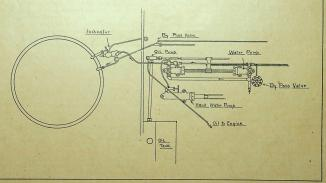
Should the fire go out on the road, shut both horner values with a short distance in order that the exhaust may draw the unburnt gas out of the burner, then stop and light the pilot with a match. Then turn on the main fire slightly, and after starting it again, it may be turned on full.
