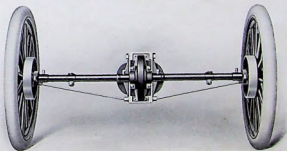
Detail of rear axle showing trussing and oil-tight casing of differential. The large elliptical case is the rear member of the oil-tight engine case.
