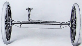
Detail of front axle, showing trussing, steering mechanism and rods; and complete protection afforded the steering gear by the axle itself. Only six moving parts in this steering gear.
