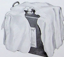
Fig. 35. Battery Covered with Wet Cloth before Lead Burning
