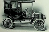
MODEL J. Limousine, scating five. 23-inch boiler and burner in front, under hood. 34 x 5 inch engine. 20 horse-power.
