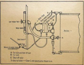
water out of it and up in the glass, thus showing that the water level in the boiler is below the indicator. Whereupon the by-pass should again be closed until the water falls in the glass again. This will indicate that the water in the boiler is above the connection "D" on the indicator.
