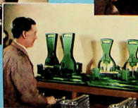
Sets of moving parts, like these connecting rods, are weighed individually to insure their uniform proper balance
