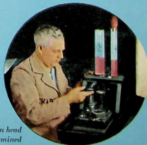
Parts bought on the outside, such as roller bearings, are also questioned. Radio amplification in this unique sound room ferrets out any noise in bearing revolution
