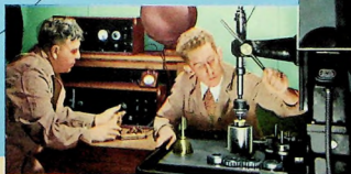
Parts bought on the outside, such as roller bearings, are also questioned. Radio amplification in this unique sound room ferrets out any noise in bearing revolution
