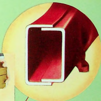
This covered box analogy is carried into the Packard frame by a wide use of box-section construction. These reinforcements, together with I-beam girders, produce a frame some 400% stiffer than conventional types
