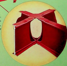
The straight-line position of the X-member's I-beam girder arms causes them to intersect the points of force application, thus increasing the resistance to twist
