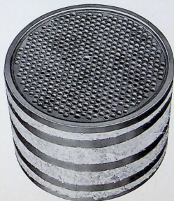
Stanley boiler. The shell and the lower head are of one piece of pressed steel. The upper head, the shell, and the ring are welded together by the oxyacetylene process. The tubes are reinforced at each end with steel bushings. The bands indicated in the cut are of thin brass, to hold in place the half-inch sheet asbestos insulation
