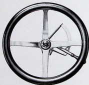
Steering wheel, showing the single throttle in the Stanley system of control locked by its locking screw
