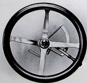
Steering wheel, showing the single throttle in the Stanley system of control locked by its locking screw; and the by-pass lever.
