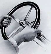
Steering wheel with hands, showing how the throttle-lever is lightly gripped in the fingers without removing the hand from the wheel.
