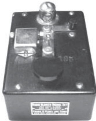
Fig. 9. Combination buzzer and blinker set: Frank B. Perry and Sons Radio Blinker Signal Set dated September 4, 1917.
