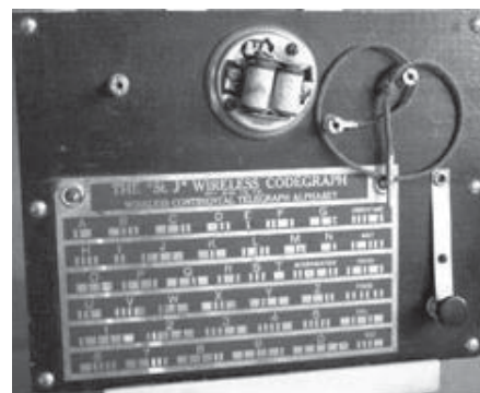
Fig. 26. “St. J.” Wireless Codegraph code plate trainer with Continental Alphabet, stamped August 13, 1912.
