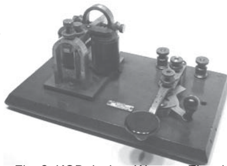
Fig. 2. KOB design: Western Electric Co. Steiner set circa 1886.
