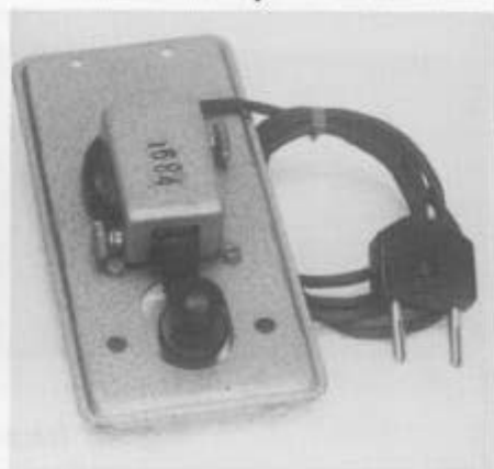
Figs. 67-68. Additional keys for the R104M
