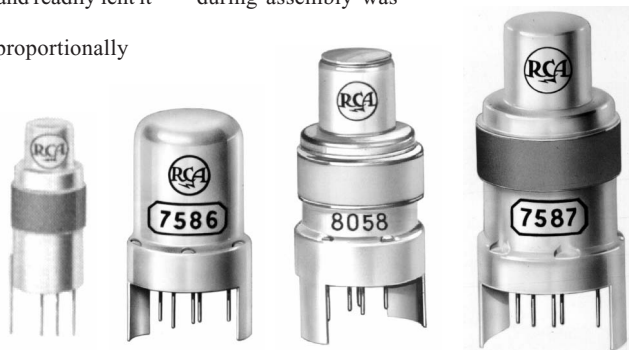
From left to right: half-size double-ended triode; 7586 single-ended triode; 8058 double-ended triode; 7587 double-ended tetrode. These are shown approximately 150% of actual size.
