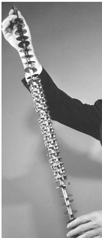
Skewer-like rods held approximately 300 Nuvistors for mass evacuation and induction heating.
