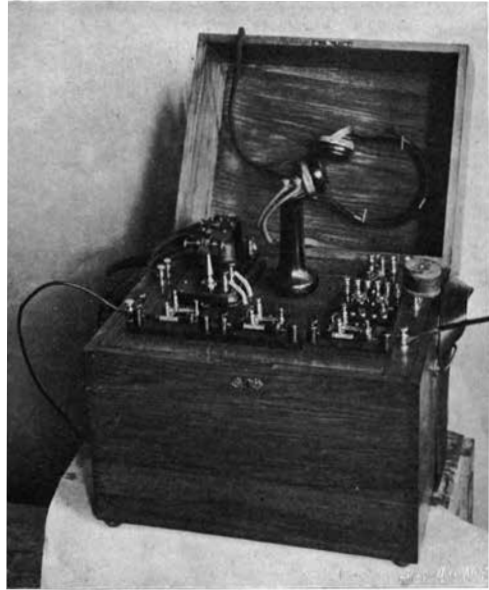
Fig. 11. This version of De Forest’s receiver with an improved “goo” responder appearing in August 1902 was said to have “greatly improved sensitiveness of the responder,” which “will respond with absolute certainty and regularity . . .” ( Scientific American , Aug. 16, 1902, p. 103)
