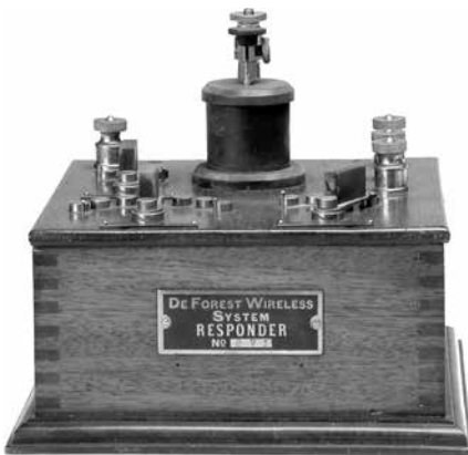
Fig. 30. An example of the De Forest liquid barretter responder in the History San Jose collection appears to be the same as the photograph of the responder taken in the De Forest tower in 1904. (Courtesy of History San Jose)
