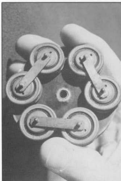
Figure 53. (left) Attached to water cooling chamber are six carbon buttons in series.
