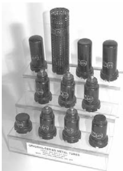
RCA's first steel-stamped metal tubes (stampings whitened for clarity). Includes both versions of the 5Z4 and the abandoned 6D5.
