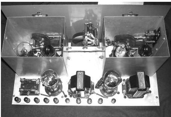
Front and back views of the AC Super Wasp with lids of shield cans removed to show construction.
