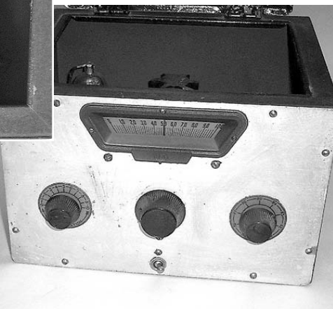
Front and cover-open top views of the 278 receiver.
