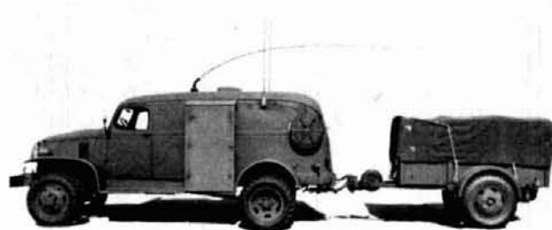
Always on the go! The SCR-399 communications truck was used to negotiate the surrender of Rommel, the "Desert Fox," in north Africa. The SCR-399 was present at the D-day invasion of Europe and accompanied General McArthur during his historic conquest of Leyte Island in the Philippines. Gasoline-powered generator is in trailer. Truck was supplied with three whip antennas for transmitting and receiving while in motion.
