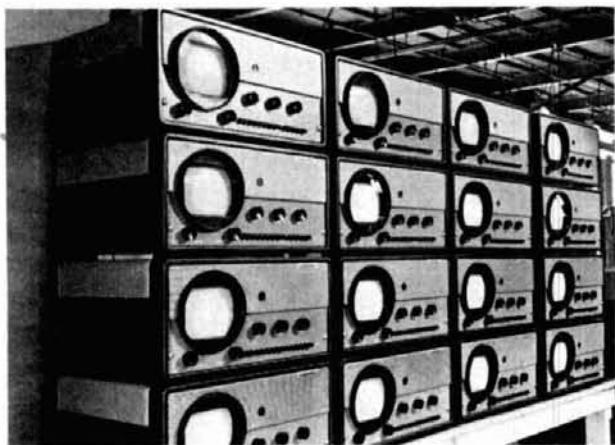
Early Hallicrafters television receivers are a collector's item now. This model had a push-button tuner that included TV channel 1, now the Amateur 6-meter band.
