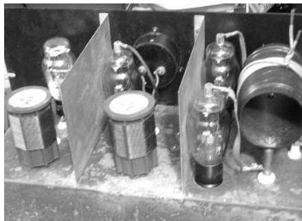
The All-Star exciter removed from the rack and sitting on author's workbench.
