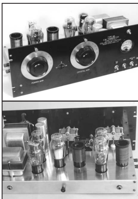
Front and rear view's of author's 4A transmitter. Note engraved ID information, black coil forms.
