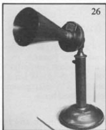
Fig. 26. WE 323 Transmitter in Candlestick Telephone with Modified Switch and "Long-Distance" Mouthpiece.
