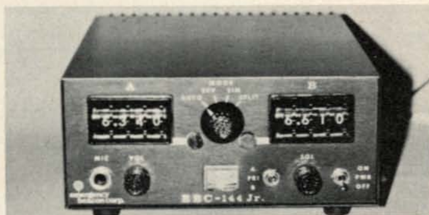
The EBC-144 JR. measures 6 \frac{5}{8} W. x 2 \frac{7}{8} H. x 11" D. excluding knobs and feet and weighs in at 6 pounds including mounting bracket. Front panel controls are self evident from the photo and are explained further in the text. The buttons on either side of the Mode switch are indicator lamps to show which set of thumbwheel switches are in use.
