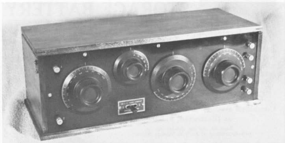
Fig. 8. The Type 220, listed by Tuska in an early catalog as the "EXPERT" TUNER. There were two wave length ranges which could be selected by use of the switch on the lower left of the front panel: 150-385 and 375-800 meters. The cost was $75.00.
