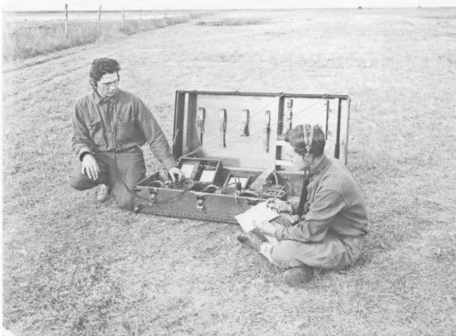
Fig. 6. Field practice copying wireless code signals using the SCR-54. At the left is the BC-14 receiver unit, and at the right a vacuum detector using a VT-1.
