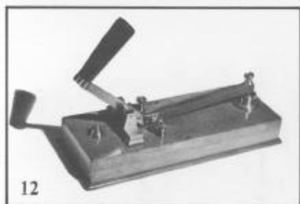
Fig. 10-13: 10. 1900 "Twentieth-Century Key" designed by Skirrow and Shirley, made by Foote Pierson Co., for operators with a "glass arm"; 11. ca 1900 submarine cable key (alternating key) with 2 levers to utilize the full curve of the alternating current; 12. "Grasshopper Key" used by Marconi and Kemp in early wireless experiments; 13. 1905 Slaby-Arco key ("Door Knob Key")—used with high-power spark transmitters.
