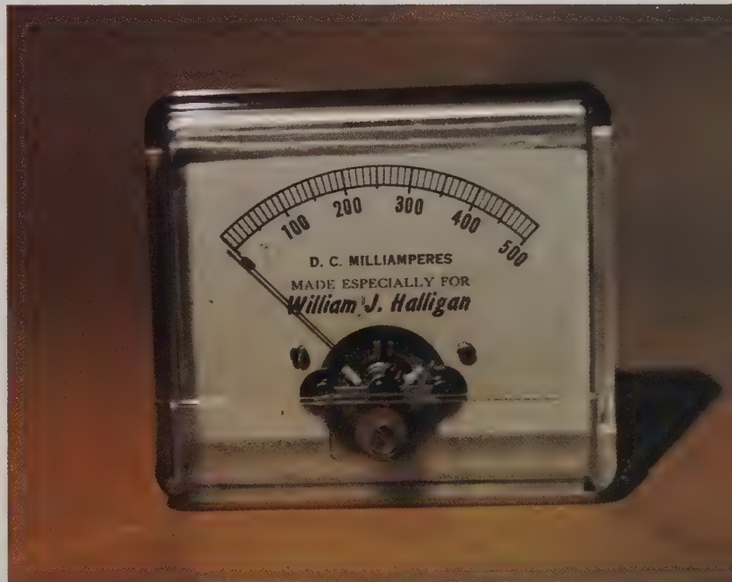
A 2-1/2" by 3" panel meter made by the Simpson Meter Co. for Bill Halligan as a promotional sample, with the hopes that Bill would chose the Simpson Co. to produce meters for Hallicrafters equipment. It dates to about 1960.
