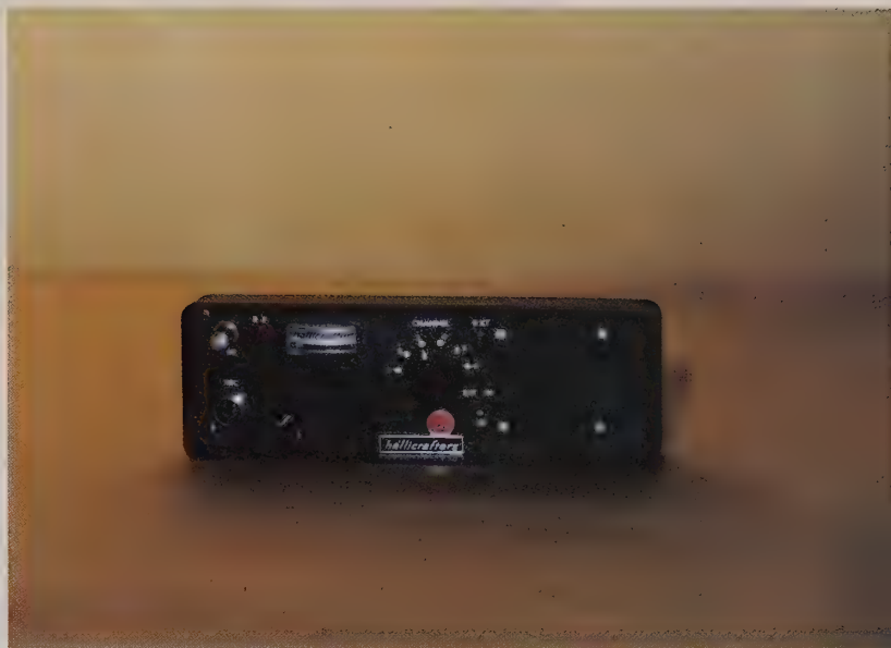
A model shop mock-up of a unknown six-channel transceiver consisting of a cardboard panel with controls and labels sitting in a steel frame, circa 1970s, from the plant in El Paso, Texas.
