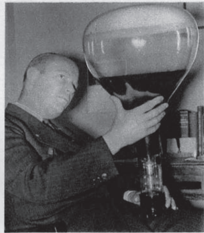
Allen B. DuMont examines the giant cathode-ray television tube he has developed. Tube has a diameter of 13½ inches.
