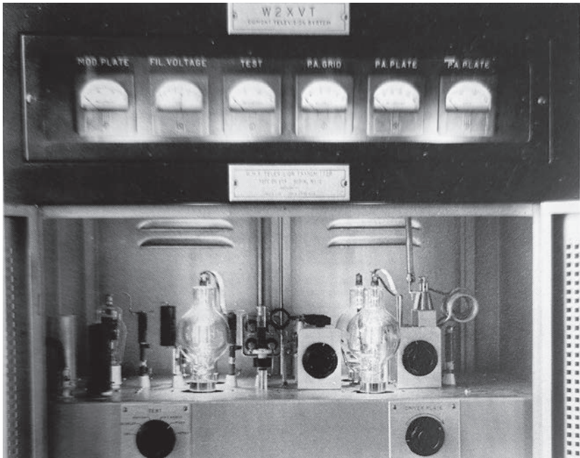
Fig. 30 W2XVT 50 watt experimental TV transmitter final amplifier stage at the Passaic factory. ( Proceedings of the Radio Club of America , Mar. 1978, p. 22)
