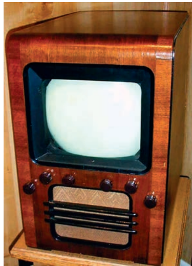
Fig. 31 DuMont Laboratories model 180 table top with 8-inch by 10-inch screen, regarded as first U.S.-manufactured TV on the market in 1938. (Early Television Foundation website)
