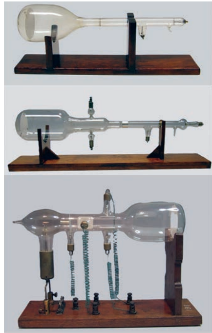
Fig. 15 Early cathode ray tube evolution. Top: early Braun tube. Center: later Braun tube with deflection plates. Bottom: later Braun tube with heated filament, known as a Wehnelt tube. (Author's compilation of photos from the Cathode Ray Tube website, www.CRTsite.com )
