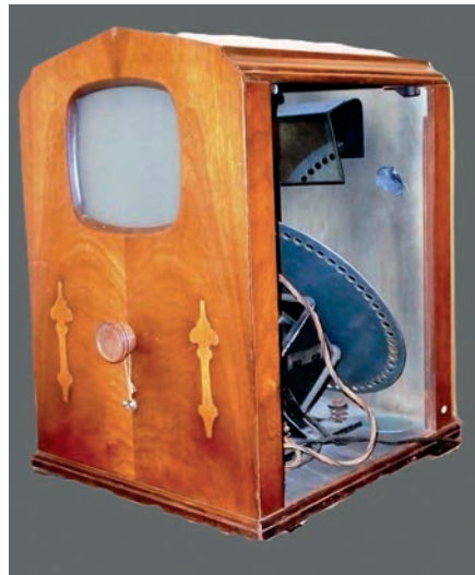
Fig. 12 Jenkins model R-400 television with lens disc and crater tube. (Early Television Foundation website: https://www.earlytelevision.org/jenkins.html )
