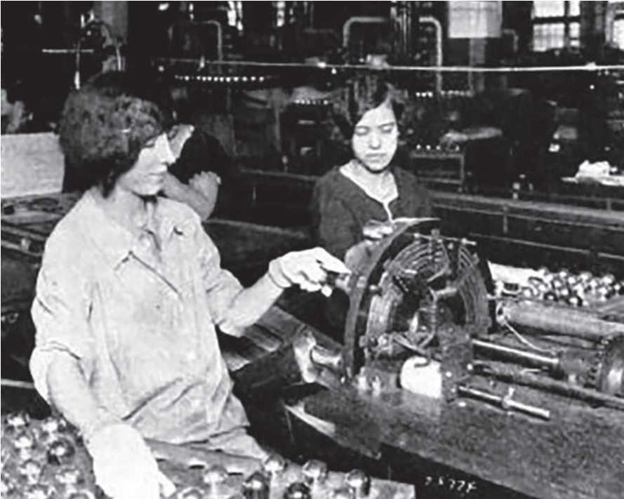
Fig. 3 Workers load tubes in an automatic tube tester capable of testing 30,000 radio tubes per day. "Here is a view of the high speed tube tester, an almost-human machine which has a capacity of 30,000 tubes a day." ( Radio Engineering , Apr. 1927, p. 677)
