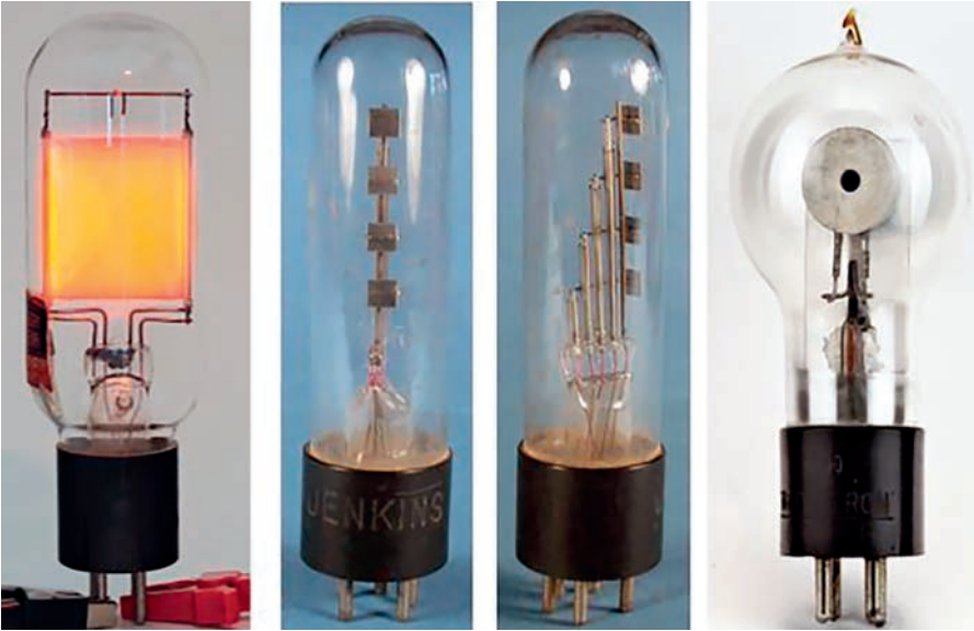
Fig. 11 Neon television tubes. Left: standard tube. Center: two 4-segment tubes. Right: crater tube. (Early Television Foundation website and author's collection)
