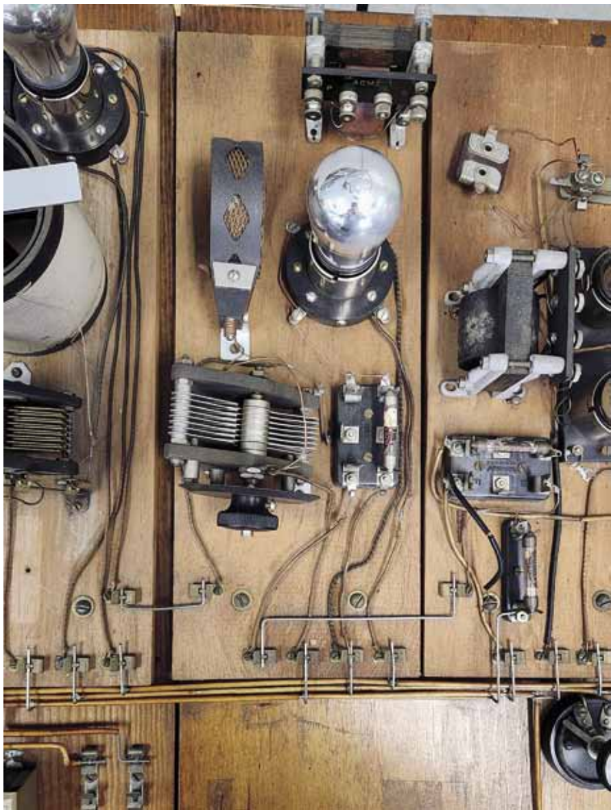
Fig. 16. The diode detector module of the Washington Receiver, as seen in the Radio Television Museum at InfoAge. (Author’s Photo)
