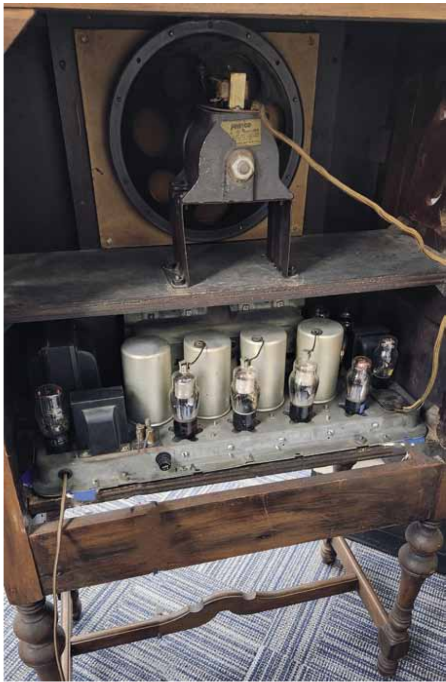
Fig. 20. Rear view of the Model 95 with the Screen Grid Plus chassis. (Radio and Television Museum at InfoAge, author's photo)
