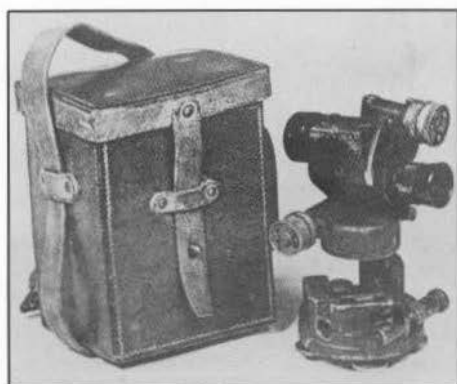
Figure 26. The AK theodolite used by the military.
