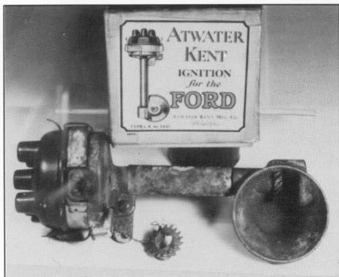
Figure 21. A retrofit ignition system for a Ford.
