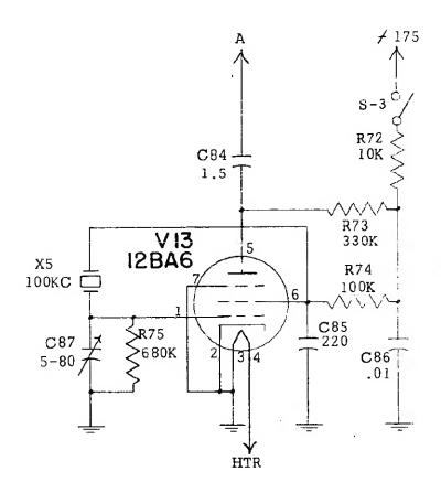
CRYSTAL CALIBRATOR SCHEMATIC DIAGRAM
