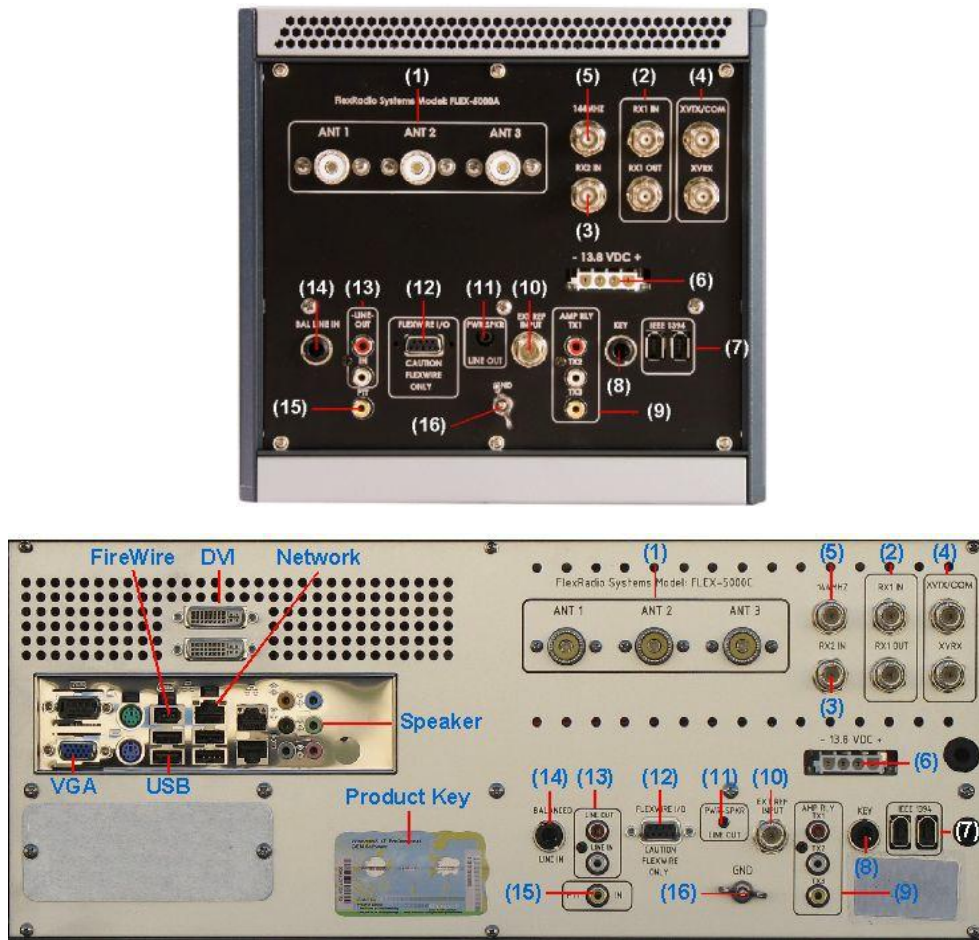
Figure 3: FLEX-5000A (top) and FLEX-5000C (bottom) Back Panel
