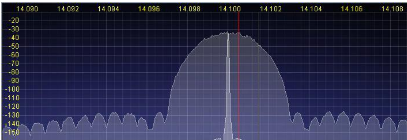
Figure 118: 25 Hz CWL Filter at 192 kHz Sample Rate/256 Buffer Size (Wide) and 48 kHz/4096 (Narrow)
