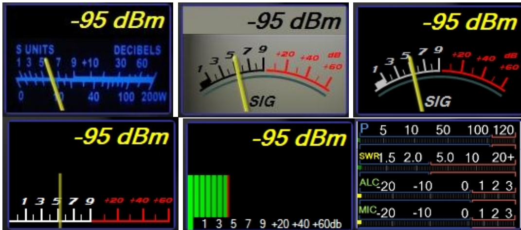
Figure 50a: Available Multimeter faces Top left to Bottom right: Analog TR7, Analog, Edge, Bar, Combo(TX2 only)
