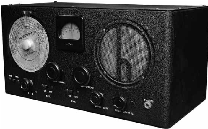
Fig. 10. Early Version of Hallcrafters S-19R Sky Buddy. All switches are slide type.
