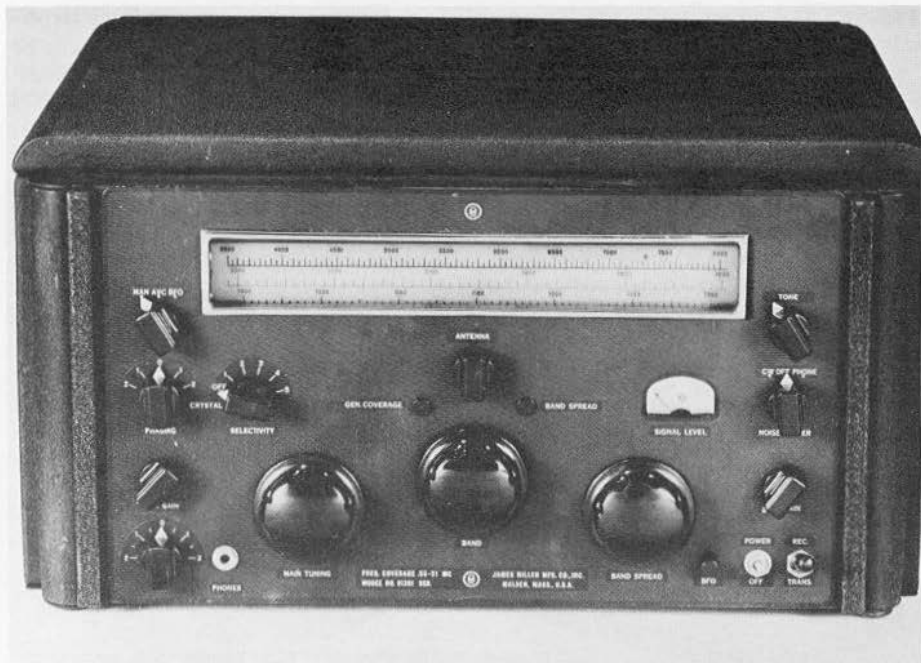
DFP (Designed For Performance) 201. Dial pointers are not shown (they were apparently never installed in this prototype). Bandspeed or general-coverage ranges are selected by interlocked push-buttons on either side of the bandswitch knob, that engage the mechanical detents on the bandset shaft.
