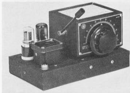
The Millen Variarm ECO (Electron-Coupled Oscillator) was ingeniously designed and worked well, but owners often sent them back to the factory to have the oscillator tube changed, a tricky procedure.
