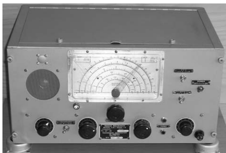
Here the radio is buttoned up in its cabinet, shock-mounted on a baseboard and ready for display.
