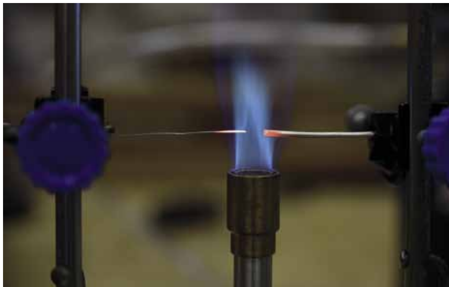
Fig. 34. This demonstration experiment with a 2 mm platinum wire inserted into the side of a Bunsen burner flame on the right and a 0.4 mm platinum wire inserted on the left shows that the temperature of the electrode depends on the diameter of the wire; the smaller diameter wire with a white incandescent glow has a temperature at or above 1300 °C while the larger diameter wire with a dull red glow has a temperature in the range of 800 °C. (Author's experiment and photograph)
