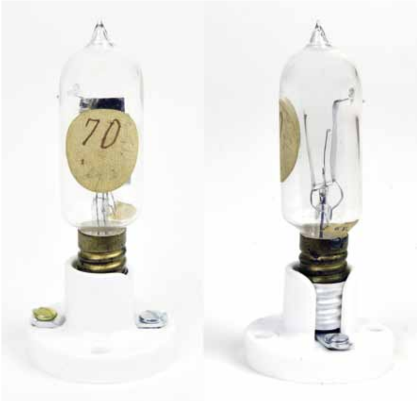
Fig. 23. This early De Forest audion dating to 1906 is one of the audions that De Forest testified “were sold to the United States Navy and tested out at the Brooklyn Navy Yard.” (Author’s collection, Provenance: Tyne/Vanicek collection)
