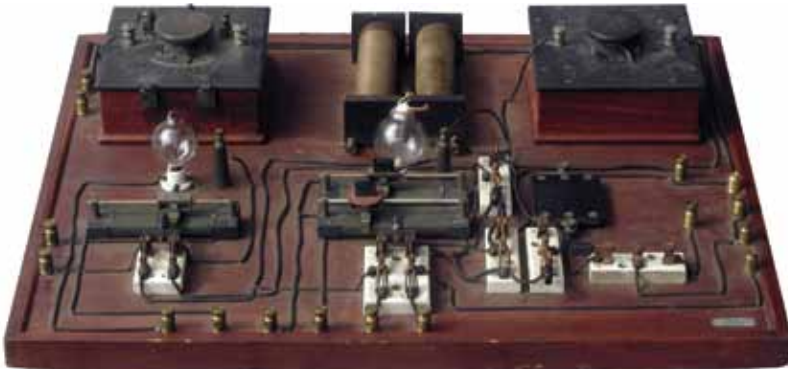
Fig. 30. Weagant used this demonstration test board to demonstrate the Fleming valve was as sensitive as the most sensitive De Forest audion configuration shown in the previous figure. (Author's collection, provenance: Edison Museum)
