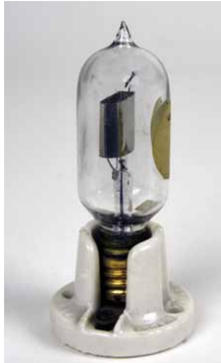
Fig. 22. This early De Forest audion bulb dating to 1906 with a "flat cylinder anode" matches the description of the audion in De Forest's testimony. (Author's collection, Provenance: Tyne/Vanicek collection)
