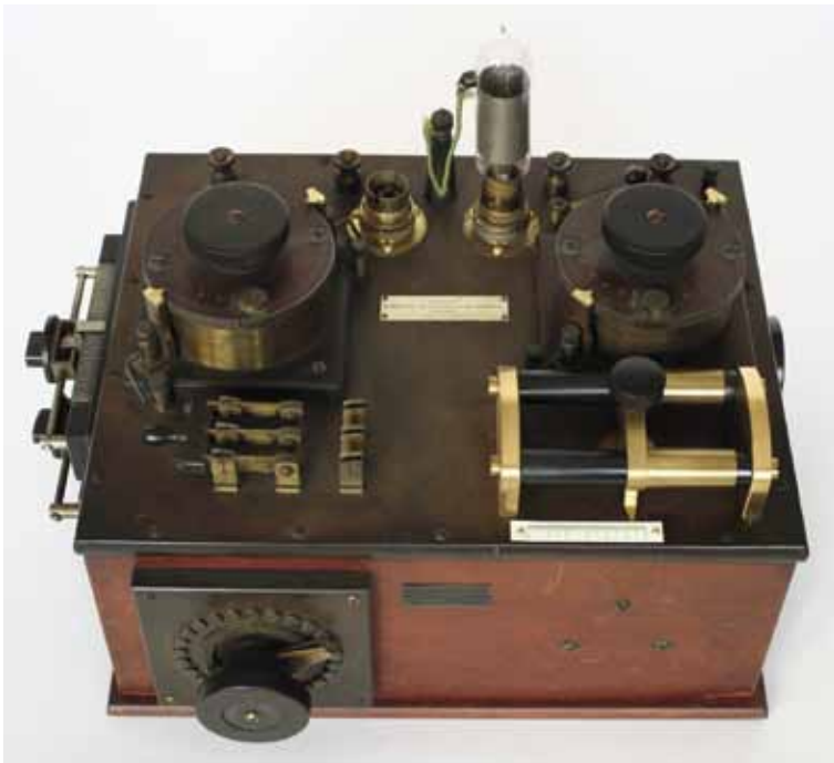
Fig. 40. Fleming's two-electrode valve with this circuit was used in the commercial systems of the American and British Marconi Companies from 1910 to the beginning of WWI. (Courtesy of Rich Groshong)
