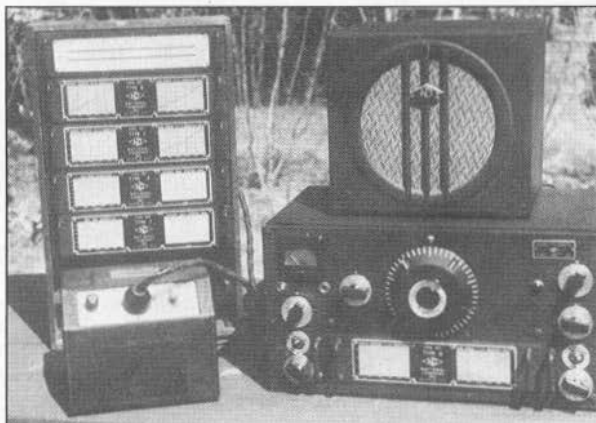
The complete set: coils, power unit, speaker, and receiver itself.
