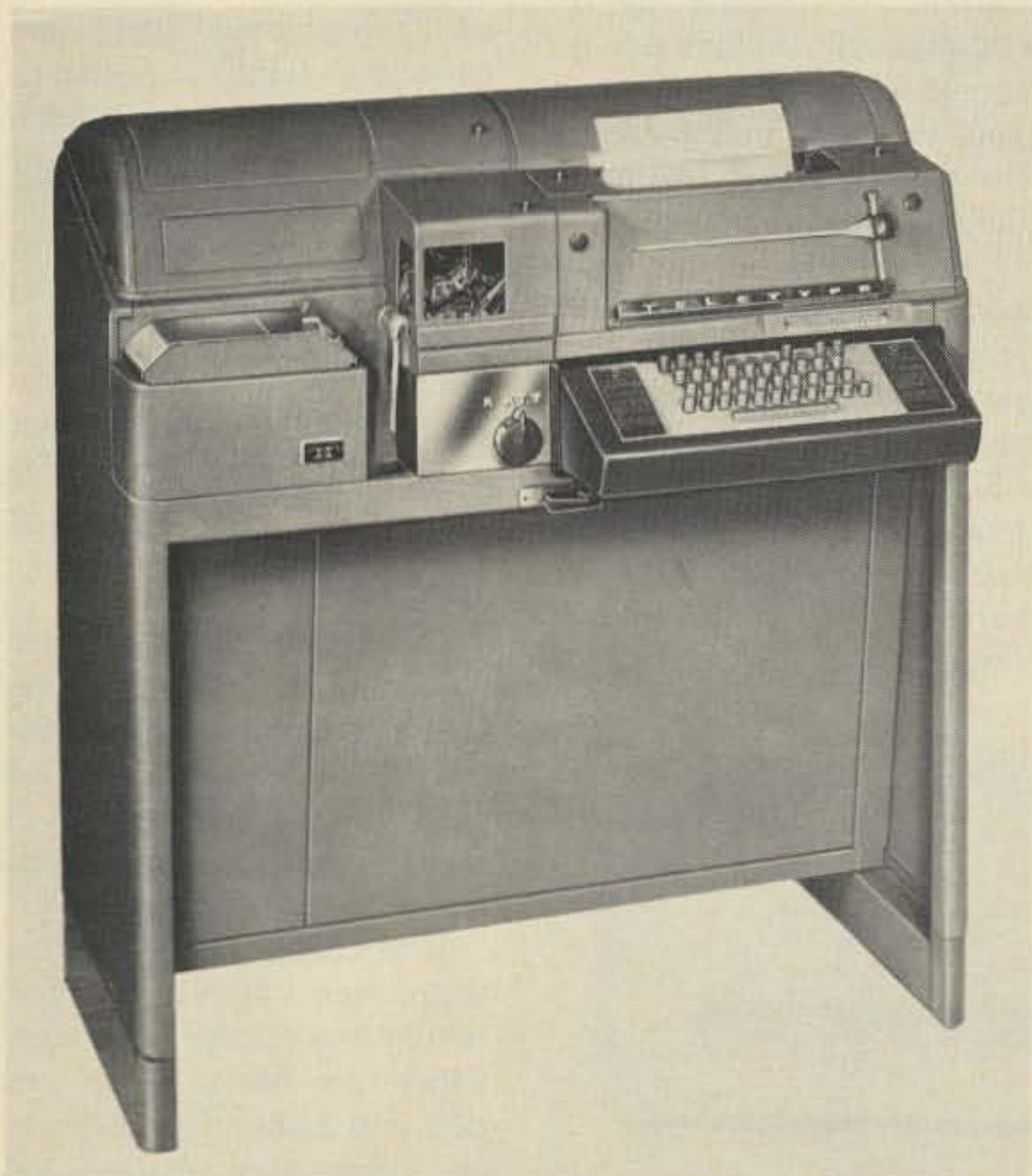
Photo 2. The Teletype Model 28 ASR shown here is a highly respected and sought-after machine. The unit includes a keyboard, a page printer, tape reader, tape punch, and a stunt box for adding special control functions. The Model 28 is built for heavy duty, 24 hour per day operation and easily operates at 100 wpm. Unlike the Model 15, the Model 28 is still manufactured by the Teletype Corporation. (Photo courtesy of the Teletype Corporation.)
