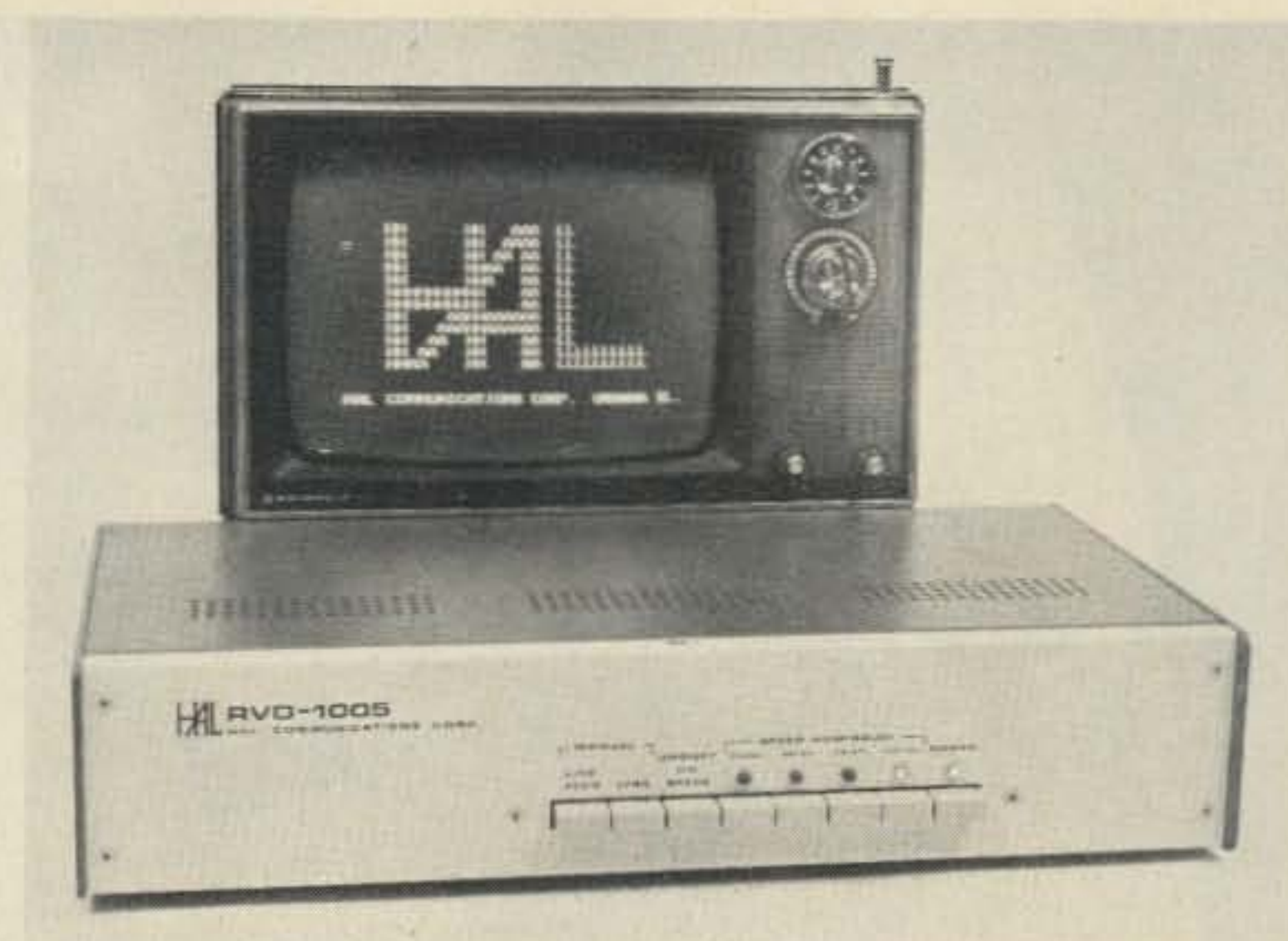
Photo 7. The RVD-1005 visual display unit is the modern answer to the teleprinter. The unit accepts demodulated Baudot signals at 60, 66, 75, and 100 wpm and displays the information on 25 lines with 40 characters per line. (Photo courtesy of Hal Communications Corporation.)
