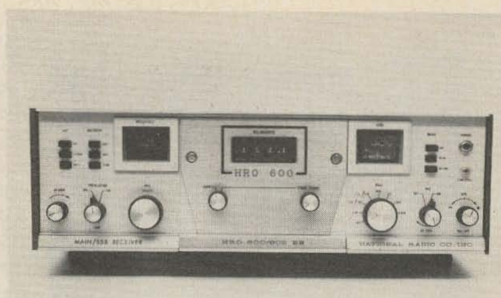
National HRO-600, a modern professional class receiver. A receiver with remotely similar performance would have occupied two six-foot relay racks in the 1930's.
