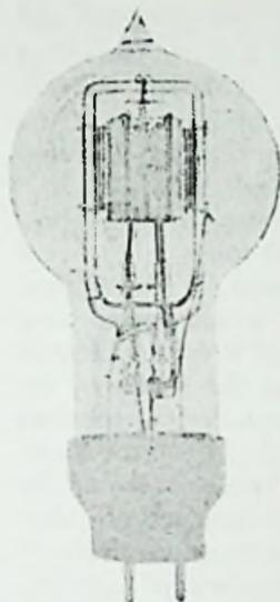
Fig. 10-7. Pilon's experimental 40-watt tube.
