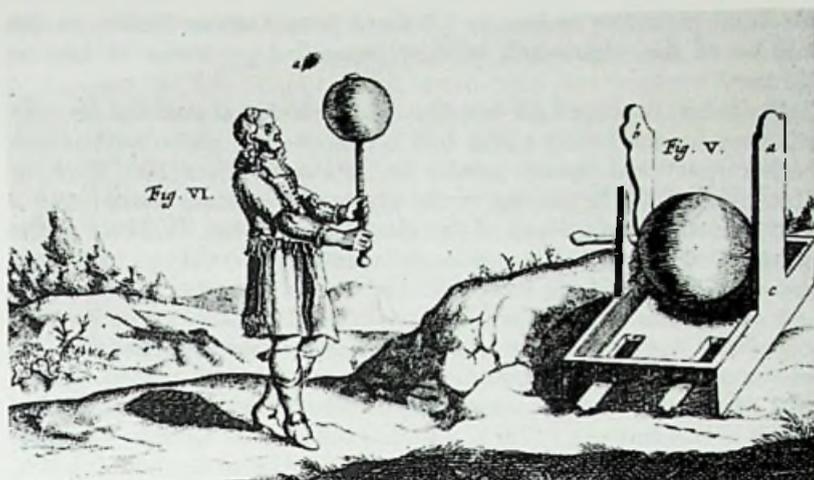
Fig. 1-1. Right: Otto von Guericke's "electrical machine." Left: operator using charged sulfur ball to repel feather. (Reproduced from *Experimenta Nova Magdeburgica de vacuo spatio*, Amsterdam, 1672.)
