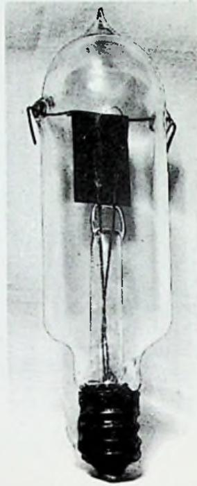
Fig. 4-13. The first grid-type Audion.
