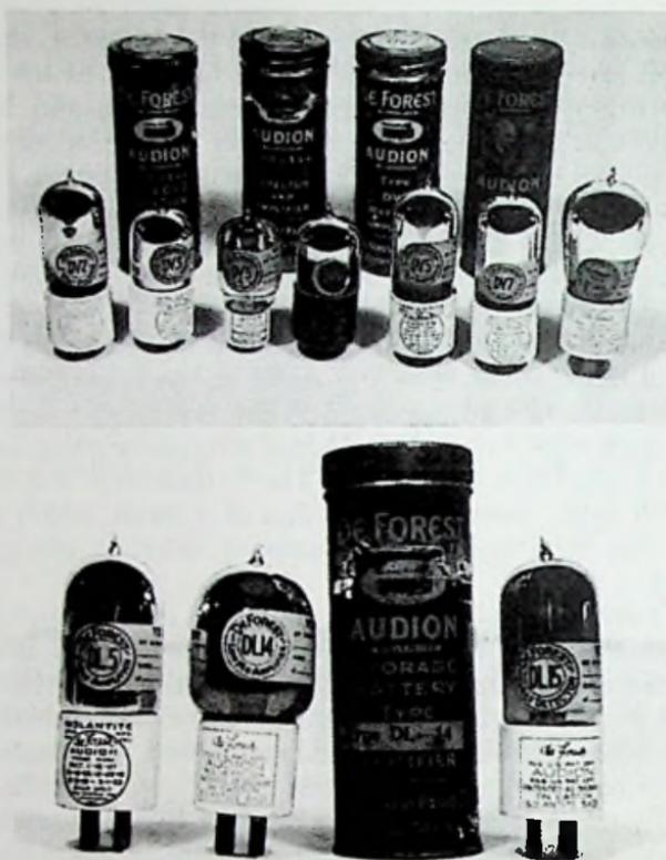
Fig. 15-1. Representative samples of de Forest tubes. In the upper row (left to right) are the DV2, DV3, DV3A, DV3, DV5, DV7, and D-01A. In the lower row, the DL5, DL14, and DL15 are shown. Metal shipping containers are shown for both series.
