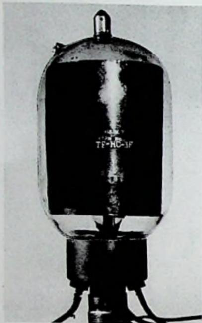
**Fig. 11-14. Round Type TF-HC-3F valve without tubulation.**
