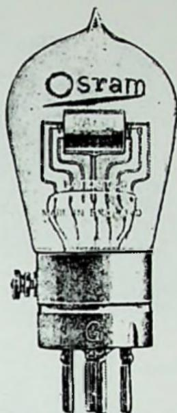
an amplification factor of 7.5 and an anode impedance of 5500 ohms. The maximum permissible anode voltage was 100 volts. It was well suited for use as a low-frequency amplifier using transformer coupling. The heater voltage of each valve was 3.5 volts and the current was 2.0 amperes. Both valves required at least a minute to become operative after being switched on.
