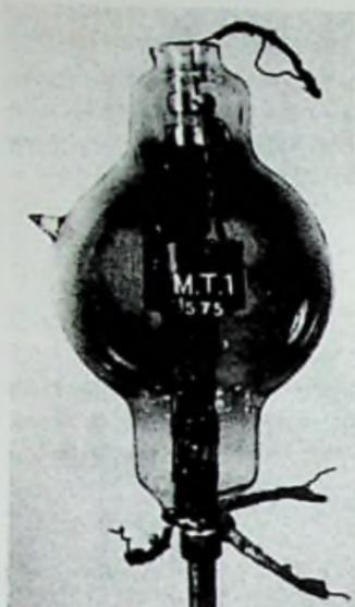
Fig. 18-20. Marconi-Osram MT1 valve.
