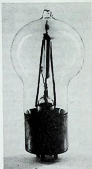
Fig. 9-18. Later version of A-P Rectifier tube.
