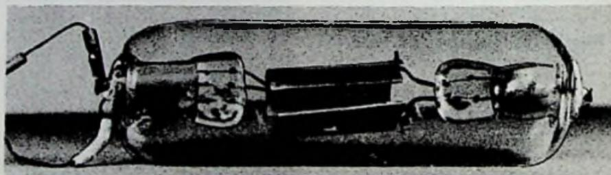
Fig. 22-17. Japanese TWW tube, showing electrode structure.
