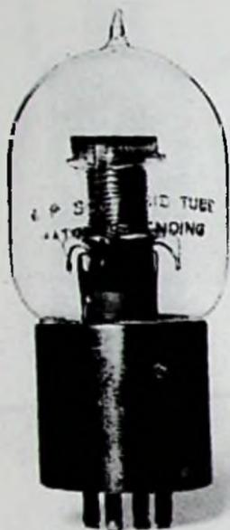
Fig. 9-20. Moorhead A-P solenoid tube.
