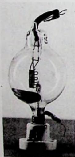
Fig. 4-19. A 1908 double-filament Audion.
