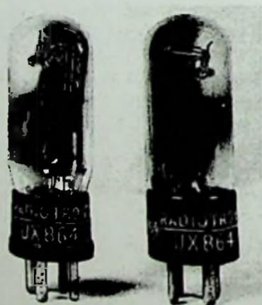
Fig. 16-27. Two versions of the Radiotron UX864: the one at the right has a low loss insulating compound in the base.
