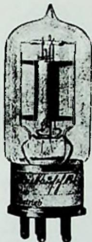
output was small, but these tubes were particularly adapted to the production of the desired gain at low anode potentials. This was essential for their use in military work, because the terminal amplifiers were self-contained portable devices operated from their own batteries. After the war these amplifiers fell into disuse, as there was no further need for the gain they produced.
