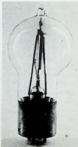
Fig. 7-6. Rectifier version of the singer-type Audion.
