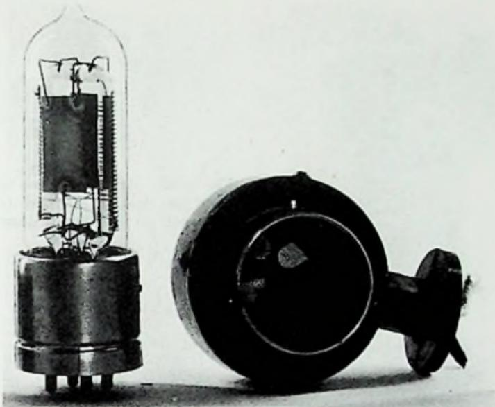
Fig. 7-16. Later type of CF-185 with four-point base and socket.
