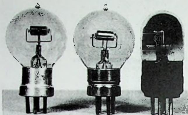
Fig. 19-3. La Radiotechnique tubes. Left to right: R3, R5, and Radio Ampli R5. The RT marking on the Radio Ampli R5 was adopted in 1923 with the change to a thoriated filament.
