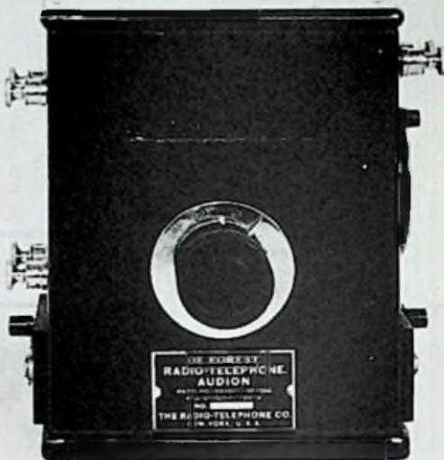
Fig. 4-18. Photograph of Audion detector in Fig. 4-17.
