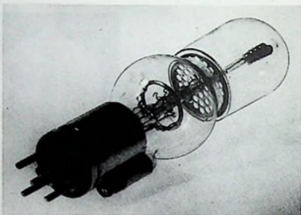
Fig. 12-6. Small LRS relay with perforated aluminum grid.
