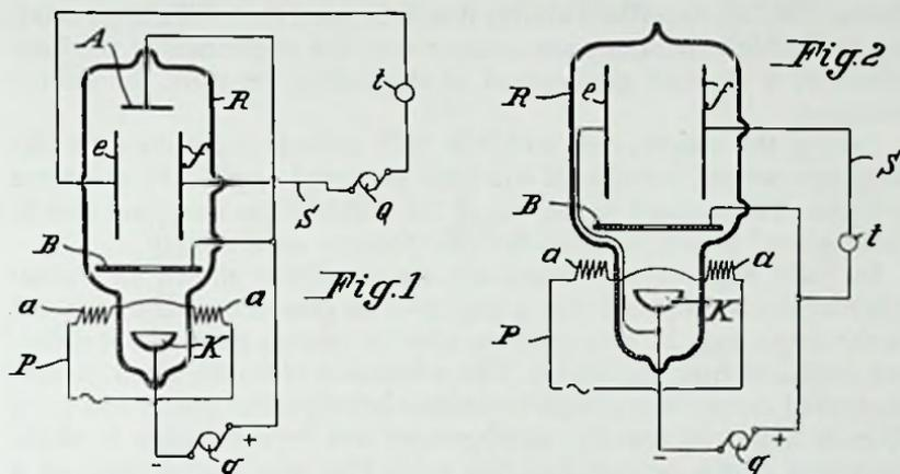
Fig. 5-5. Von Lieben gaseous cathode-ray relay of 1910, using magnetic deflection of the cathode-ray beam acting as "ionizer." (Reproduced from D.R.P. Nr. 236,716.)
