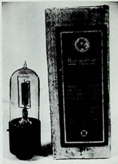
Some of the earliest Westinghouse tubes were stamped on the base "Manufactured for the Radio Corporation of America by Westinghouse Lamp Company U.S.A." in addition to the Westinghouse emblem etched on the glass. These tubes also had the word Radiotron in an arc rather than in a straight line parallel to the base. Even after the practice of etching the maker's name on the glass was discontinued, this arched marking continued to be used.
