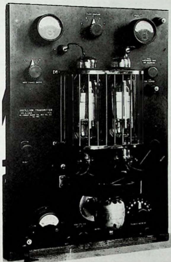
Fig. 7-26. Oscillation transmitter Type OT200, using two 500-watt-input tubes.
