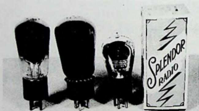
Fig. 20-17. Splendor tubes. Left to right: V1508, G450, and HF.
