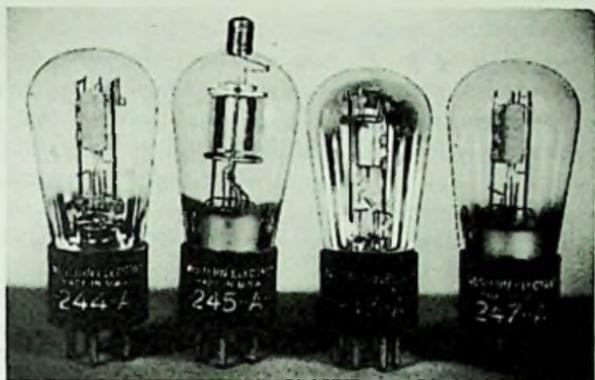
Fig. 14-33. Indirectly heated cathode Western Electric vacuum tubes. Left to right: 244A triode, 245A tetrode, 247A early type with solid anode, 247A later type with mesh anode.
