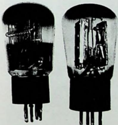
Fig. 22-13. Tungram PP430 and PV495 tubes.
