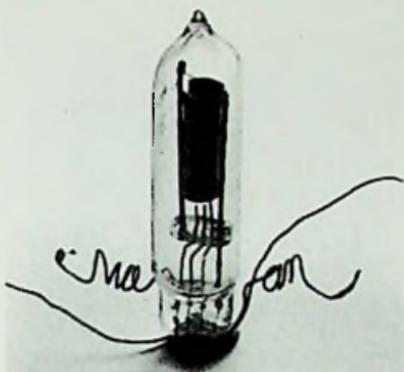
In 1927 the 239A (Fig. 14-28), a modification of the 215A, was introduced. It was equipped with a small UX base and a sturdier element structure for applications where low response to mechanical shock was all-important.
