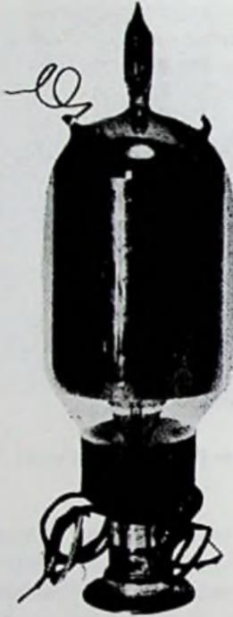
Fig. 11-10. Round Type T valve with multiple cathodes.
