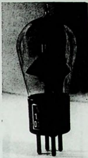
shown in Fig. 21-42. The U60 took a filament current of 0.06 ampere at 1.1 volts. Its amplification factor was 8.5, mutual conductance 350 micromhos, and anode impedance 24,000 ohms. No electrical data on the UL550 are available. This company ceased to exist in 1930, and its rights went to Telefunken.
