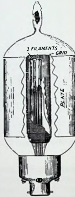
Fig. 11-11. Drawing of the internal structure of the Type T with multiple cathodes.
