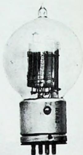
Fig. 6-22. The final form of the VT-2, Navy CW-931 vacuum tube. Note the phenolic insert in base.
