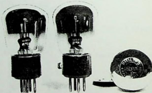
Fig. 20-10. Variants of the Philips E415 tube. Left to right: five-pin base, four-pin base and side connection, top marking.
