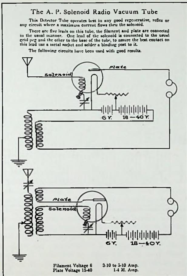
Fig. 9-21. Instruction sheet for the A-P solenoid tube.
