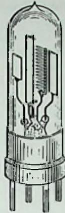
The S.T. Co. Ltd. was founded and operated by John Scott-Taggart. The formation of this company was announced in an advertisement on October 20, 1926.<sup>51</sup> The valves they sold were marked ST, followed by significant numbers; the first digit indicated the filament voltage. Valves ST21, ST22, and ST23 had 2-volt filaments; ST41, ST42, ST43 had 4-volt filaments; ST61A, ST61B, ST62, and ST63 had 6-volt filaments. These valves were advertised on February 26, 1927.<sup>52</sup>
