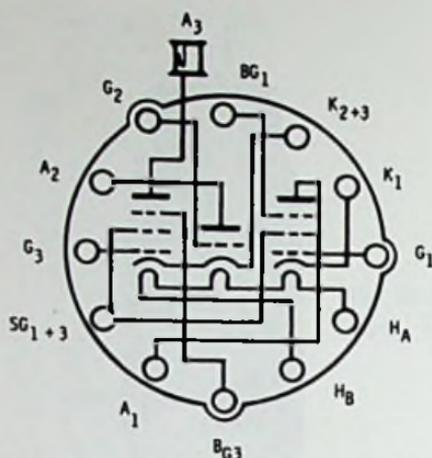
Fig. 21-34. Base connections of Loewe WG36.
