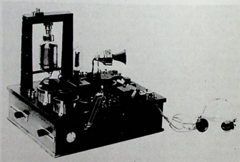
**Fig. 11-15. Marconi short-distance wireless telephone transmitter and receiver. The valve in the gallows frame is the Round Type TN, used for transmitting. The one at the right rear is the Round Type C used for receiving.**
