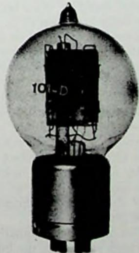
Fig. 14-1. The earliest type of 101D repeater bulb, 1921.
