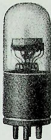
Fig. 12-45. C.H.F. Müller receiving tube.
