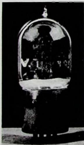
Fig. 9-14. The Marconi VT with steel-stamped base markings.
