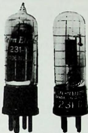
Fig. 14-29. The 230D vacuum tube. Fig. 14-30. The 231D vacuum tube.
