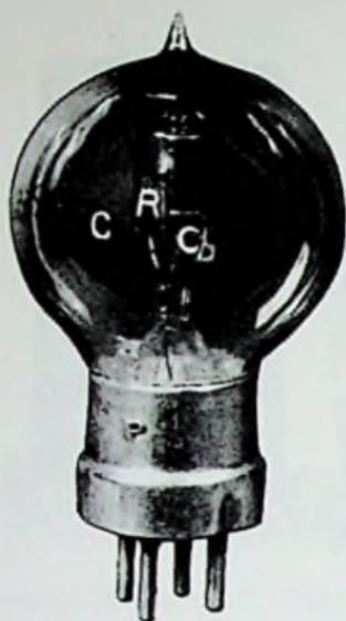
**Fig. 18-39. Radio Communications Company Polar R valve.**
