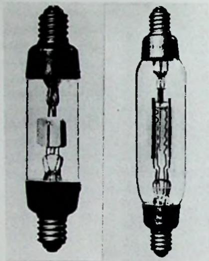
Fig. 13-3. N.V. Bal detector tubes, 1918. The one at the left is the earlier construction.
