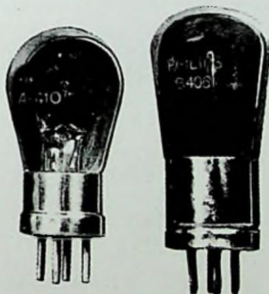
Fig. 20-8. Philips A410 and B406 tubes.
