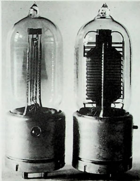
Fig. 6-20. The final form of the VT-1 vacuum tube.
