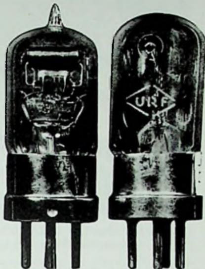
with 0.5 ampere. The recommended anode voltage was 30-75 volts. Two samples of the D II are shown in Fig. 20-5; the one with the tip is the earlier version.
