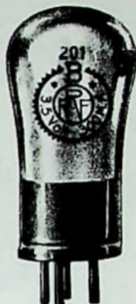
micromhos, and the anode impedance 9000 ohms. Most of the later Huth tubes carried the trademark HUTH with the letters interlocked.
