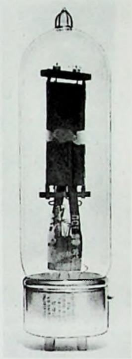
Fig. 14-18. The 214A vacuum tube.
