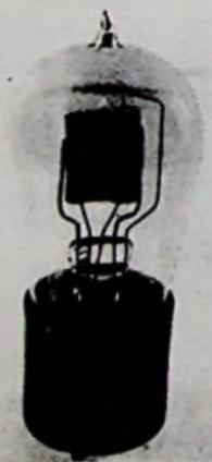
Fig. 16-15 (Left). An experimental Westinghouse rectifier or Fleming valve.
