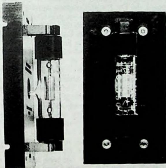
Fig. 17-1. Front and side views of RAC3 Audion in mounting socket.
