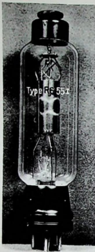
Fig. 21-20. Telefunken RS551 low-power transmitting tube.
