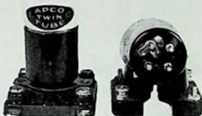
1.1 amperes at 3.0 volts for the heater. When operated with 90 volts on the anode and grid bias of  $-4.5$  volts the anode current was 4.6 milliamperes. Under these conditions it had an amplification factor of 8.5. The anode resistance was 9100 ohms, and the mutual conductance was 935 micromhos.
