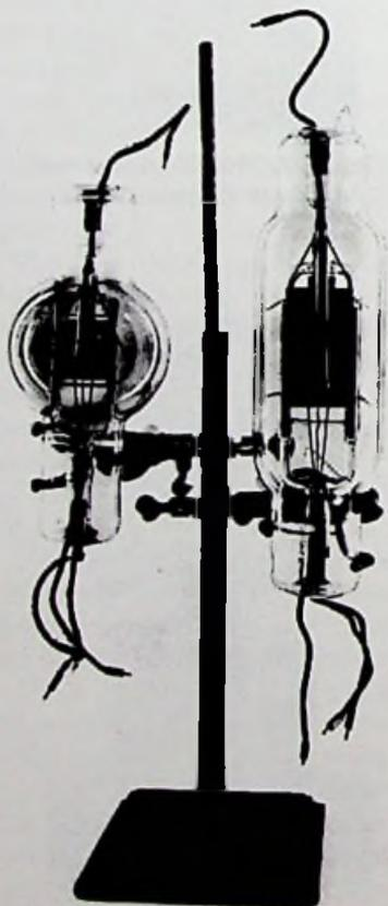
Fig. 7-25. Early 250-watt and 500-watt (input) Oscillions.
