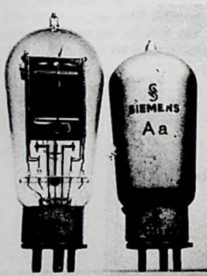
Fig. 21-12. Siemens & Halske Types Da and Aa tubes.
