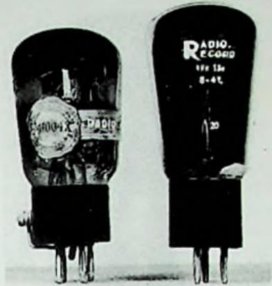
In 1927 they began to manufacture tubes, adopting the brand name Radio Record. Two of their tubes are shown in Fig. 20-18—the RRR134 is a half-wave rectifier and M1004X is an output amplifier.
