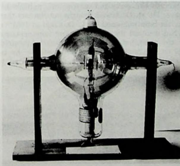
**Fig. 8-9.** The tube used by Alexanderson to modulate a small high-frequency alternator in wireless tests between Schenectady, New York, and Pittsfield, Massachusetts, in 1914.
