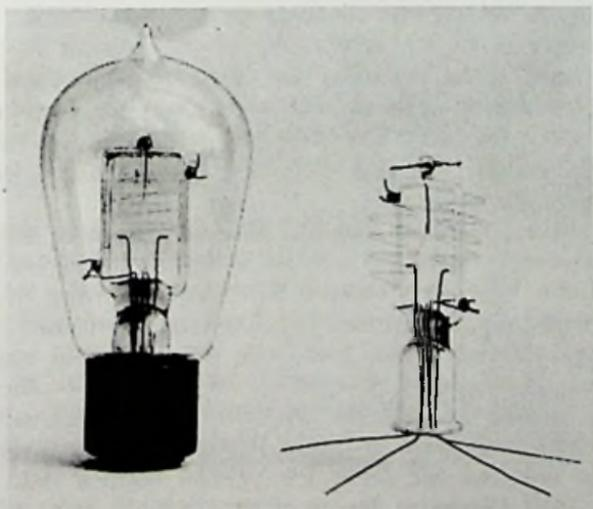
Fig. 8-7. Type CA Pliotron, vintage 1918. Left: completed tube. Right: element assembly on stem.
