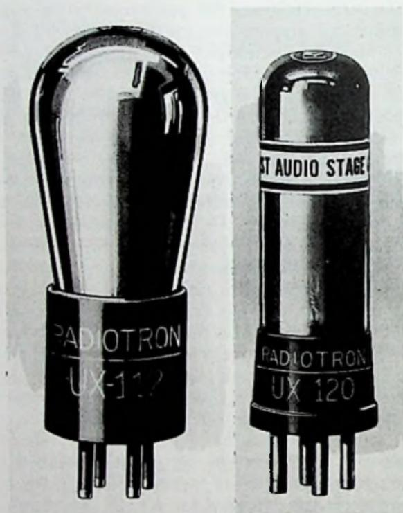
Fig. 16-7. Radiotron UX112 and UX120 tubes.
