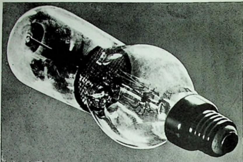
Fig. 5-7. Von Lieben electrostatically controlled cathode-ray relay of 1910.
