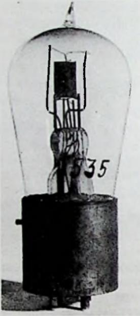
Fig. 8-20. The VT-13, or later Type CG-890 tube.
