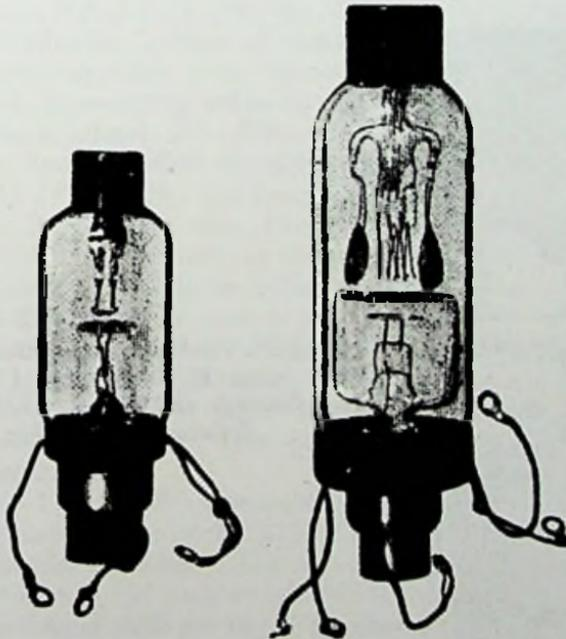
Fig. 12-24. Telefunken EVN94 (left) and EVN129 (right) tubes.
