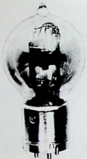
Fig. 6-21. An early form of the Type E, 205A, or VT-2 vacuum tube. This tube has a sheet-metal, wax-filled base.
