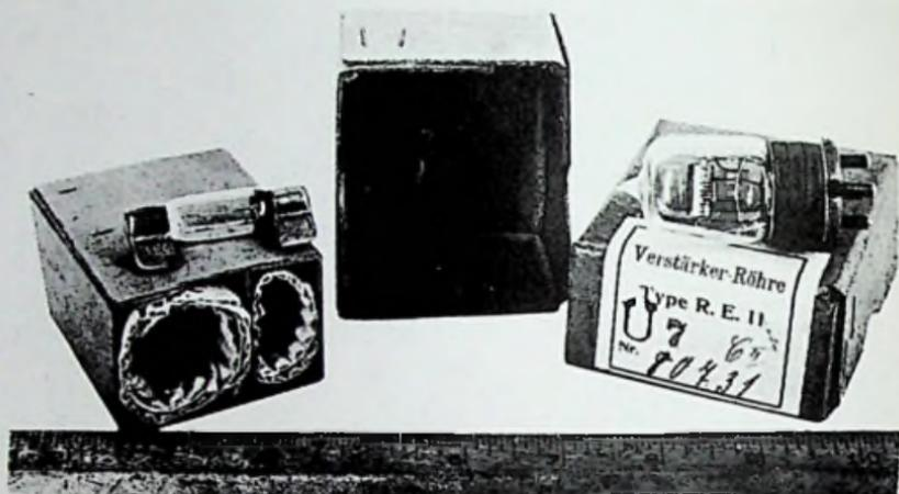
Fig. 12-29. The RE11 tube with ballast resistor.
