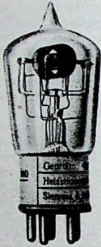
Fig. 12-18. Siemens & Halske 110 tube. (Reproduced from *Veröff. NachrTech.*, 1935.)
