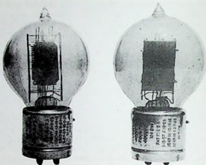
Fig. 14-9. The 102DW and 104DW vacuum tubes.
