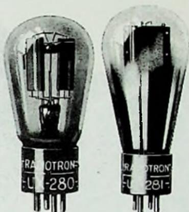
the same filament conditions as the UX213; that is, 2 amperes at 5 volts. The filament emission was in excess of 400 milliamperes. The rated maximum output current was 125 milliamperes, almost twice that of the UX213. The maximum recommended ac voltage per plate was originally 300 volts but was later increased to 350 volts. In order to assist in the dissipation of heat and reduce the tendency toward back emission, the anodes were carbonized.
