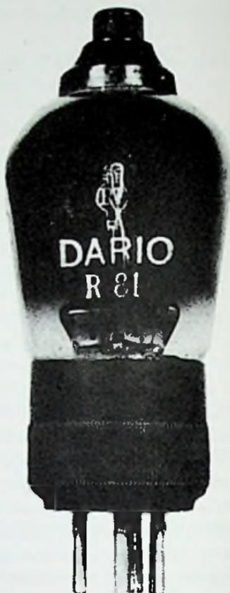
Fig. 19-11. Dario R81 radio-frequency tetrode amplifier.
