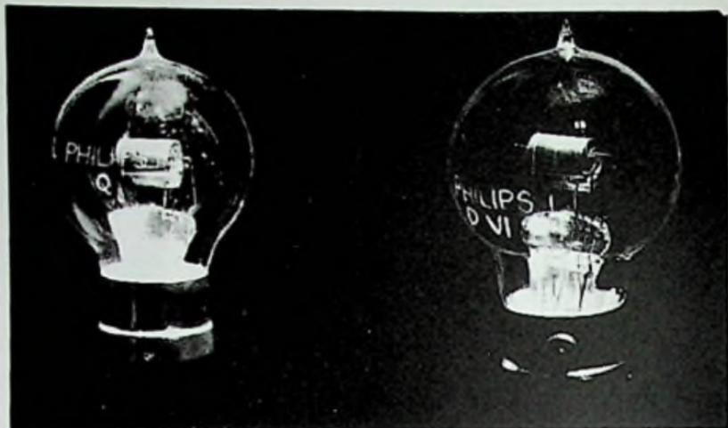
Fig. 20-6. Philips Q and D VI tubes. Tubes are the same but bear different markings. The Q is the earlier marking.
