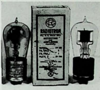
ucts of work done in the Research Laboratory of General Electric and were being sold for amateur and experimental use only. In the UV designation U signified that it was an apparatus unit and V that it was a vacuum tube. This system of significant tube coding broke down rather soon. In the first RCA catalogue, dated September 1921, there was offered for sale the UV712 Audio Frequency Intervalve Transformer.
