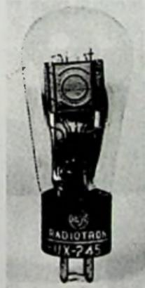
Fig. 16-14. Radiotron UX245 tube.
