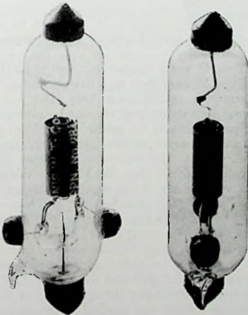
Fig. 11-27. Two views of the Marconi V24 valve.
