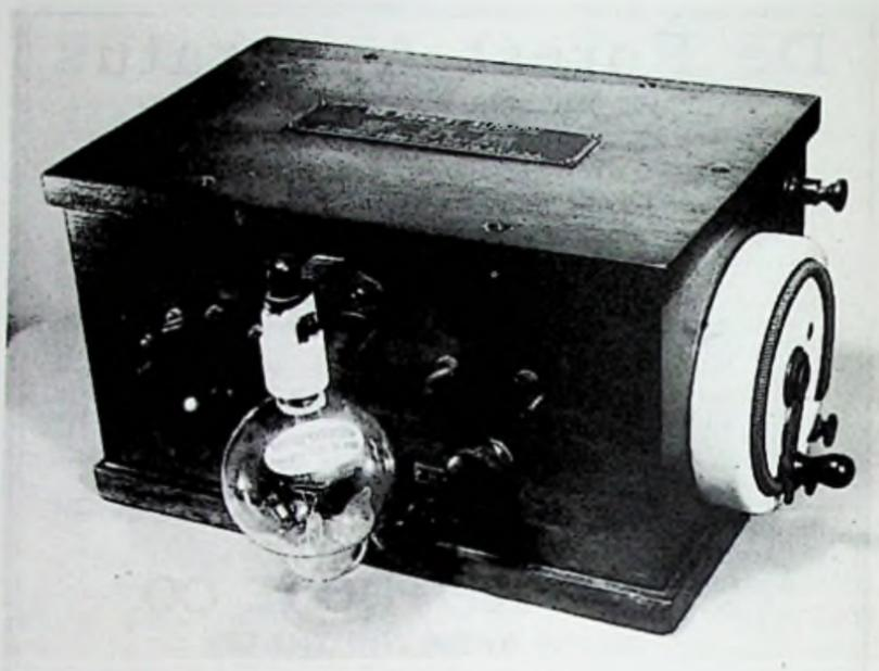
Fig. 4-23. The RJ4 detector. The tap switch at the left controls the plate voltage, that at the right is the off-on switch for the filament. The filament rheostat is mounted on the right-hand end of the box.
