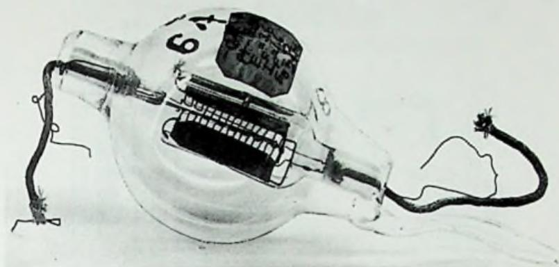
Fig. 6-6. Type A telephone repeater element.
