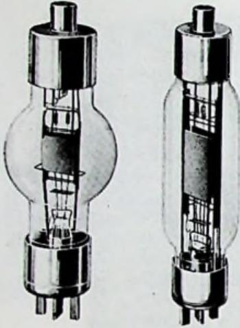
Fig. 7-27. The 250-watt-input Type 1D and 500-watt-input Type 1C Oscillions, vintage 1920, equipped with end fittings.
