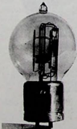
**Fig. 6-16.** A 101B repeater bulb with the arbor welded to the stem below the press.
