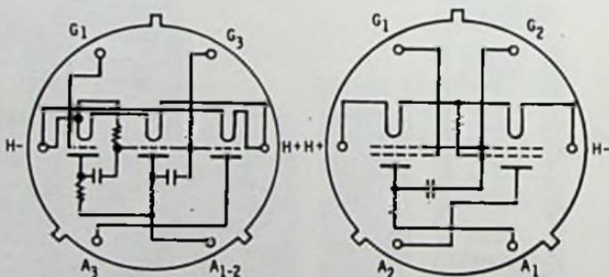
Fig. 21-31. Base connections of Loewe 3NF (left) and 2HF (right).
