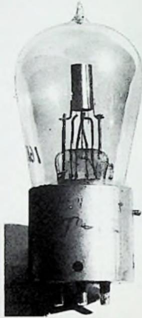
Fig. 8-21. Type T Pliotron; Signal Corps VT-12.
