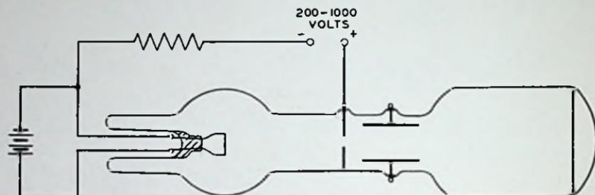
Fig. 5-1. Wehnelt's Braun-type tube with oxide-coated hot cathode.
