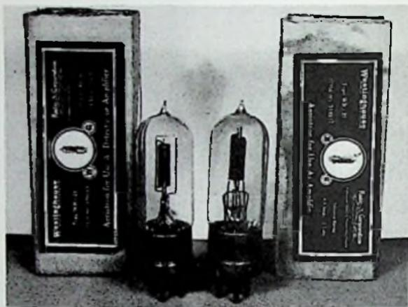
Fig. 16-4. Westinghouse E. & M. Co.'s Aeriotrons WR21D and WR21A, with packing cartons. The 21D, with lacquered tip, is at the left.
