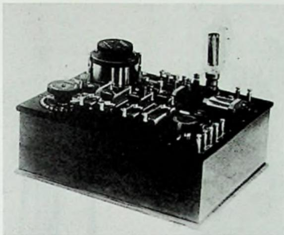
Fig. 11-9. Marconi Type 27 receiver (1914-1918) using Round Type N valve.
