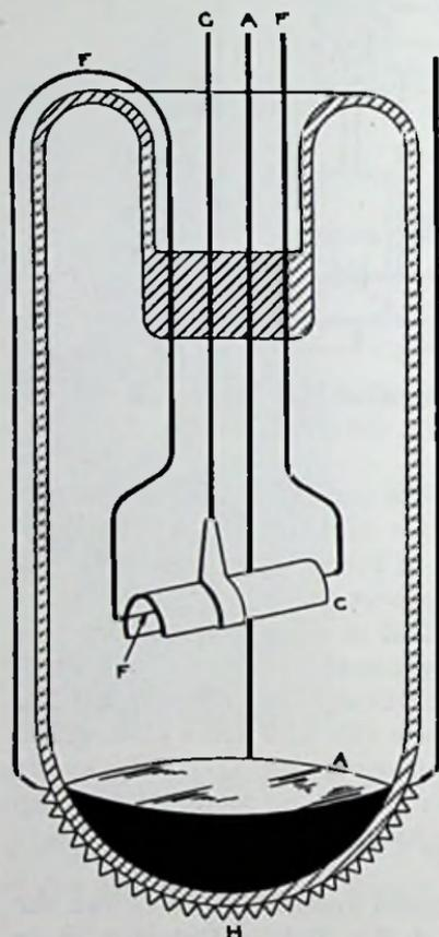
Fig. 17-9. Diagram of an early Sodian detector. (Reproduced from *Proc. I.R.E.*, Apr. 1923.)
