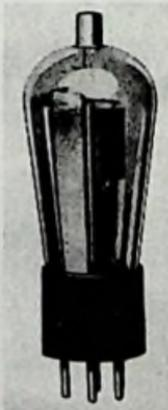
Fig. 16-13. Radiotron UY224 tube.
