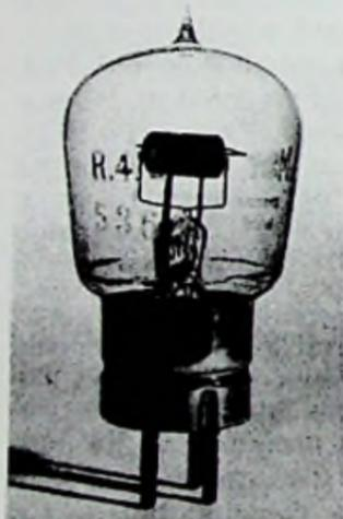
Fig. 18-17. Marconi-Osram R4B valve.
