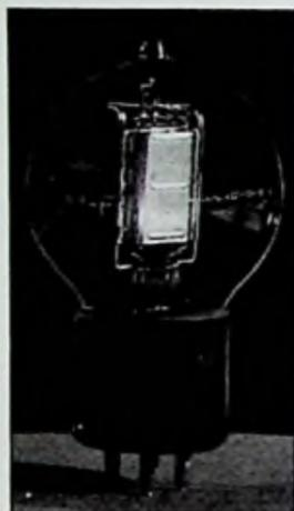
Fig. 14-5. The earliest form of the 101F vacuum tube.
