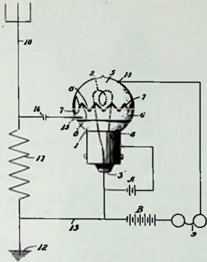
formed a part is described in an article in *QST* for October 1921.<sup>12</sup> The circuit in which it was used is shown in Fig. 17-8. The filament operated directly from a 6-volt storage battery and was insensitive to voltage changes. In the detector the tube was surrounded by a coil through which direct current flowed, setting up a magnetic field parallel to the axis of the tube. The statement is made that the tube "must be tuned to the desired signal." This was accomplished
