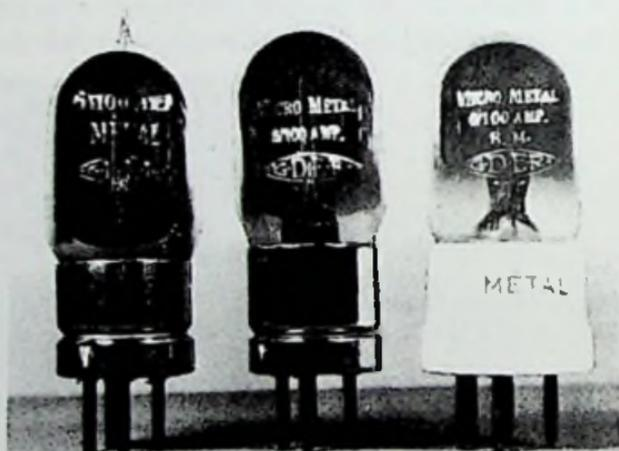
Fig. 19-4. Variants of 6/100 Micro-Métal. The tube at the extreme right, "MICRO-METAL 6/100 AMP. R.M.," was intended for operation with ac on the filament. Note G·D·E·R· markings.
