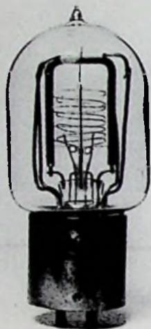
Fig. 8-8. Later sample of the Type CA Pliotron with cylindrical bulb and Shaw standard base. This tube has an improved electrode structure.
