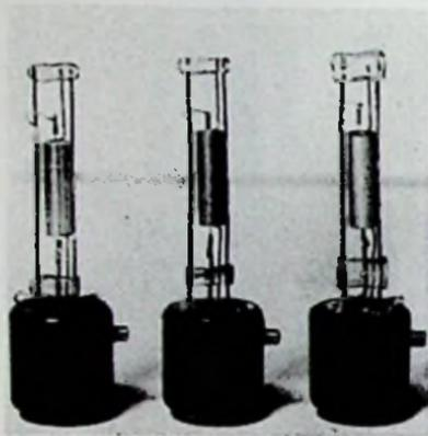
Fig. 14-26. The 215A vacuum tube with glass envelope removed. This illustration shows the increased size of the stiffening glass bead and the molded bayonet pin.
