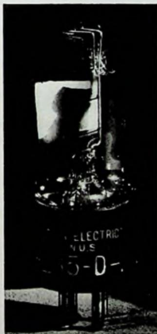
Fig. 14-31. The 221D and 235D vacuum tubes.
