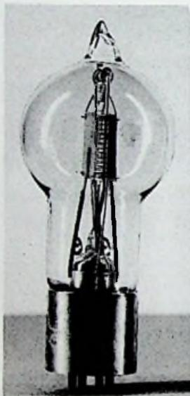
Fig. 7-5. Final construction of the singer-type Audion.
