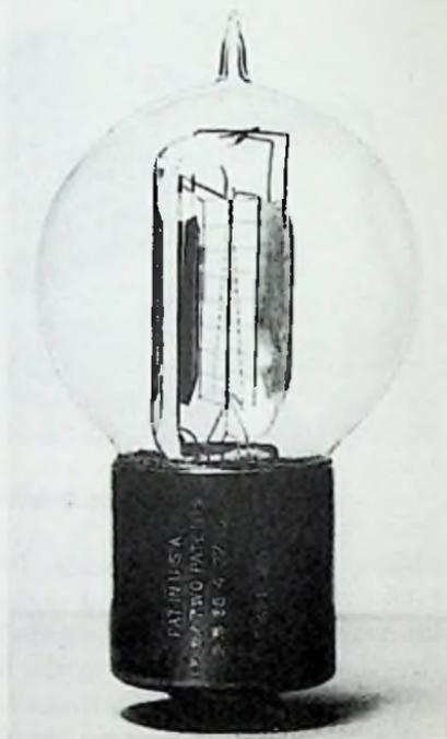
Fig. 6-8. Type M telephone repeater element, later coded the 101A repeater bulb.
