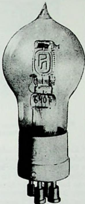
Fig. 13-4. Russian PR1 tube. (Reproduced from *Gedenkenboek N.V.V.R.*, 1926.)
