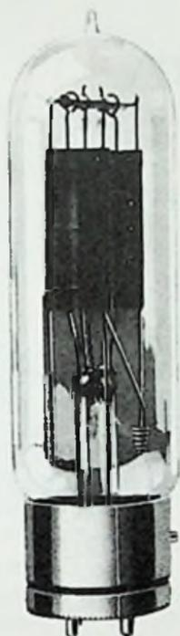
Fig. 16-23. Radiotron UV204 tube.
