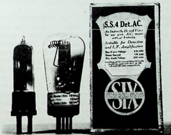
Fig. 18-31. Six-Sixty valves. Left: early design with no specific designation. Right: SS4 Det. A.C., made by Mullard.
