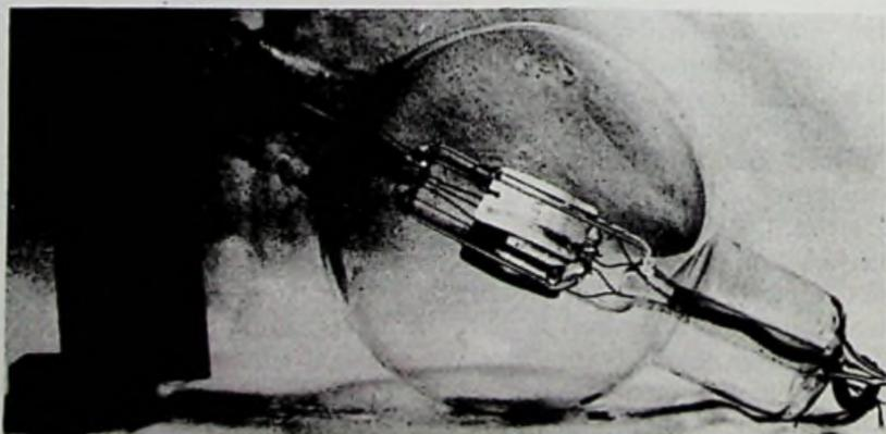
Fig. 7-9. A high-power Oscillation, vintage of 1915, 50 watts input.
