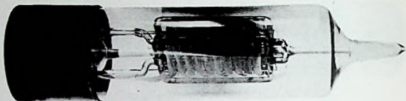
Fig. 6-29. The Type S or 204A vacuum tube.
