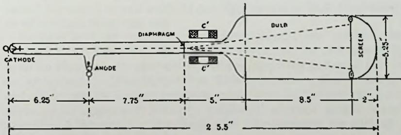
Fig. 4-25. Ryan's tube, as made by Müller-Uri.
