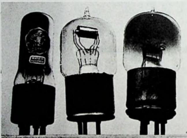
Fig. 22-9. Triotron tubes RS4, SV7, SV10.
