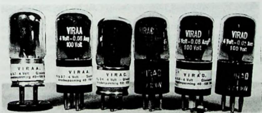
Fig. 20-19. VIR tubes. Two samples each of VIRAA, VIRAC, and VIRAD, showing variations in markings.
