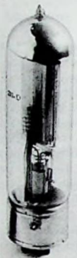
Fig. 14-13 (Right). The 211D vacuum tube with metal base.
