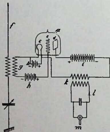
Fig. 12-2. Von Bronk arrangement for using de Forest Audion as a high-frequency amplifier. (Reproduced from D.R.P. Nr. 271,059.)
