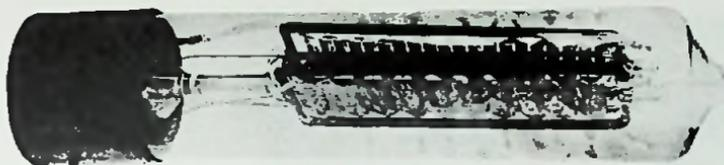
Fig. 6-27. The Type W, or 204B vacuum tube.
