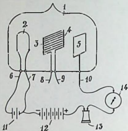
Fig. 13-7. Majorana's electronic deviator. (Reproduced from D.R.P. Nr. 281,014.)
