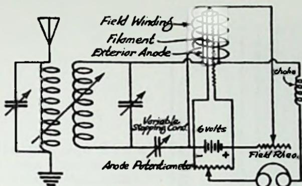
Fig. 17-8. Circuit in which the Connecticut J117 tube was used.
