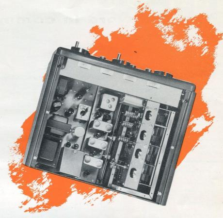
Top view showing front-end unit with shield removed (right), the IF strip (center), and the audio, BFO, crystal calibrator, and power supply unit shown together (left). Chimney-type shield on rectifier provides means of exhausting heat through rear of cabinet.
