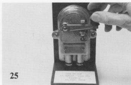
Figs. 18-25. 18: Heavy-duty keying relay from the spark era, 1914; 19: Stromberg-Carlson buzzerphone for use in trenches, WW I; 20: W.E. trench buzzerphone, 1917; 21: J-5 flameproof key with "mitten" knob for use in open-cockpit aircraft, 1917; 22: J-7 flameproof key, combined with a light-signaling device, 1917; 23: Early French oil key for spark use; 24: WW I Marconi key; 25: Yard-arm blinker key, 1911.
