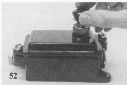
Figs. 49-52. 49: Swedish army key; 50: KMK-2 South African military key; 51: WW II German Baumuster T-1 military key; 52: WW II British Admiralty key.
