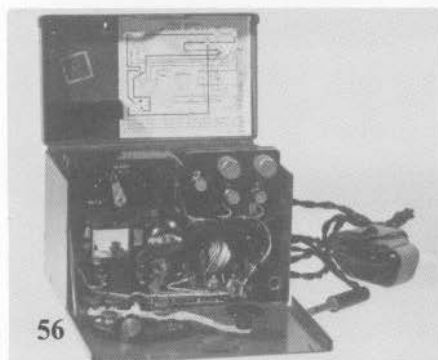
Figs. 54-57. Miscellaneous keys not referred to in the text: 54: 1900 Double-lever Bunnell Cable Key, used by the military in Spanish-American War; 55: 1920s Logan SpeedX, adopted by U.S. Navy for CW operation; 56: 1941 J-41A, complete telegraph station for field operation; 57: 1941 J-51, for use with a light-signaling device.
