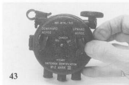
Figs. 41-44. 41: WW II keys, British Army and RAF; 42: RAF WW II "bathtub" key; 43: RAF light-signaling key, WW II; 44: 1941 J-37 U.S. military key...steel lever and leaf spring on a dielectric frame; could also be designated J-41A, J-43, J-44, J-45, J-46, J-47.
